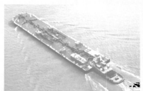
ATB unit, Tug, Capt. Fred Bouchard and Barge B. No. 275 departing the New Orleans area with the first load of product as an OPA'90 compliant unit following the double-hulling of the barge at Bollinger Gulf Repair. (Photo Courtesy of Bollinger Shipyard)
