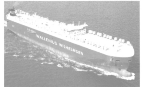
MV Tamesis is a new generation Mark IV RoRo ship with a groundbreaking design. The Mark IV RoRo provides 35 percent more covered capacity for specialized RoRo cargo than the previous Mark III design.
