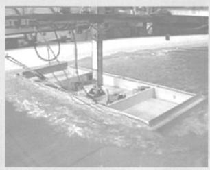
Pulling a model of the cable ferry sideways. Note the yellow cords simulating the cables to the trolley. (Courtesy Vizon Scitec with permission)
