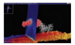
3002, extends the functionality of multibeam echo sounders to cover three-D imaging of biomass and other acoustic reflectors that might be present in the water column. 160 acoustic beams are sampled digitally with a spatial resolution of 15cm for each ping, creating a digital image of a slice of the water mass under the transducer.
