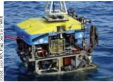
Positioning System (SHARPS) to Woods Hole Oceanographic Institute. SHARPS is being used for positioning and control of the 6,500 m Jason/Medea ROV during missions where very high resolution position information is required.
