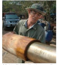
C.S. Inter Marine's shipyard manager Khun Patum Sardsiri checks fit of tamarind shaft bearing.
