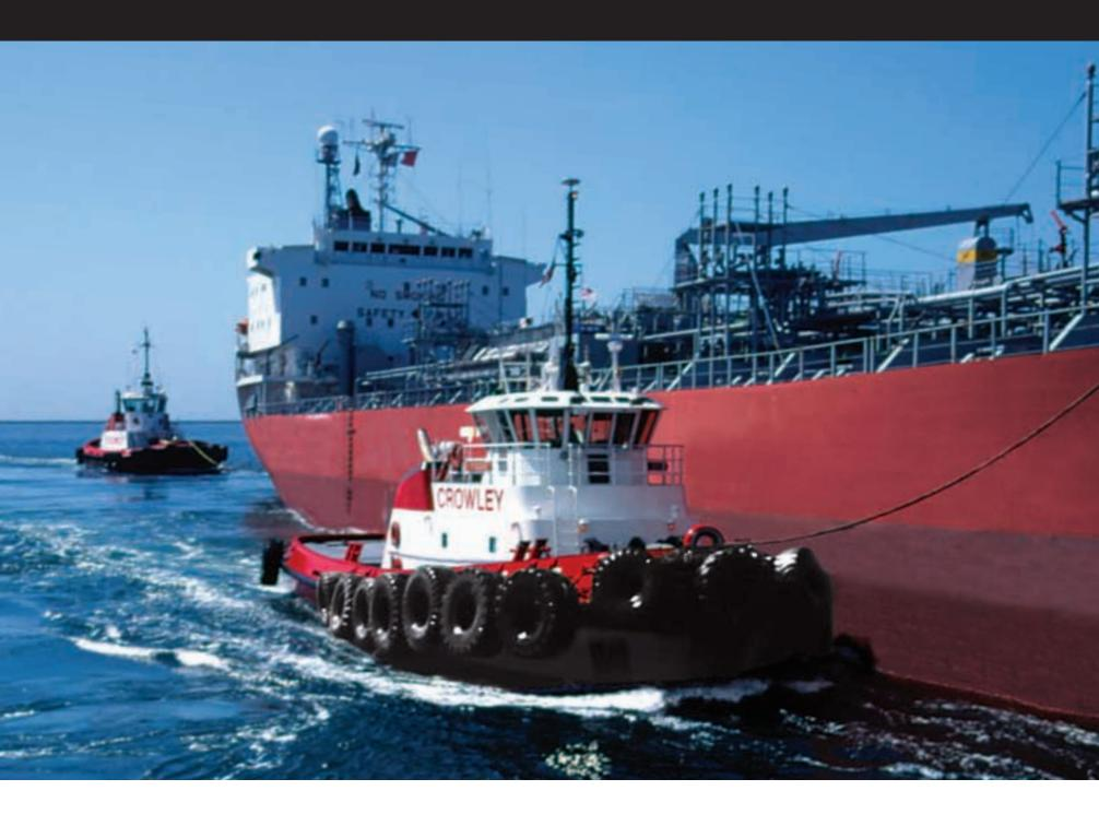
When it comes to ship assist and escort services, Crowley's got you covered. After all, we operate the most advanced fleet of tractor tugs on the West Coast. Like our Harbor Class tugs, built with custom-designed skegs for precise steering and control. And cycloidal propulsion units for a 360-degree thrust. They can go from full-power-ahead to full-power-90-degrees in just 11 seconds. With moves like these, it's no wonder our safety record is unparalleled.
