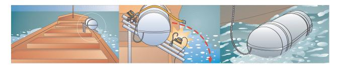
The Hammar remote release systems are designed to release heavy loads, such as liferafts or other objects, with little effort on all kinds of vessels. Two remote release systems are available:
