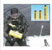
ed by the pinger receiver which can be carried by a diver or deployed from a boat.
