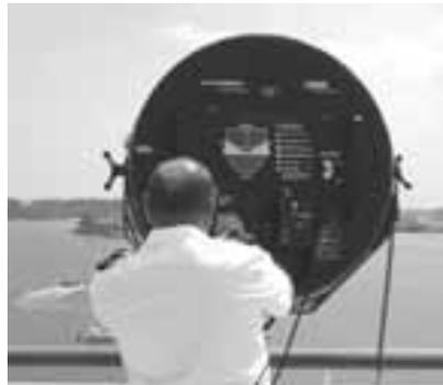
The Long Range Acoustic Device (LRAD) creates a directed acoustic beam that is clearly audible and intelligible beyond 500 meters.
