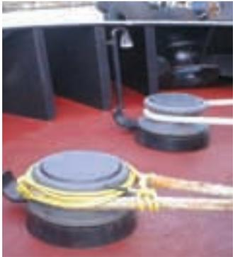
Schoellhorn-Albrecht Machine Co. has developed a new line of roller fairleads using state-of-the-art composite rollers to protect soft, synthetic rope from wear caused by traditional steel rollers. The composite material combines high strength, low water absorption and the
