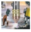
deliver high-speed, low-cost standard plasma cutting; high-quality precision cutting and marking; and high-current, thick-plate cutting all with a single plasma torch. When configured for 600-amp operation, the system can cut and mark material from 20 ga. to 6.25 in. (1mm to 160mm) with uniform quality.
