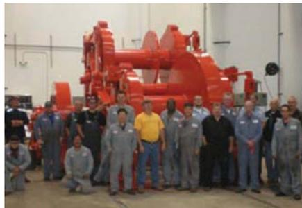
tons of line pull. The anchor handling drum features a drive consisting of four hydraulic motors installed on a modular, removable gearbox for ease of maintenance. The escort drum is a completely independent, modular winch powered by two additional hydraulic motors and is capable of 10.3-tons of line-pull and speeds up to 85 m/min. The escort drum's
