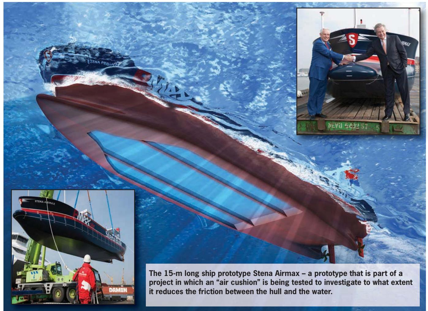
The 15-m long ship prototype Stena Airmax – a prototype that is part of a project in which an “air cushion” is being tested to investigate to what extent it reduces the friction between the hull and the water.
