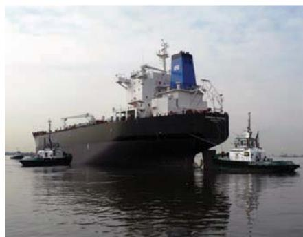
pleted by 2011. The 46,000 dwt vessel was floated off of its blocks and was transferred by tug from the Building Dock to the Outfitting Dock. When completed, the 600 ft. Overseas Martinez will be sold to American Shipping Company and bareboat chartered to OSG America.
