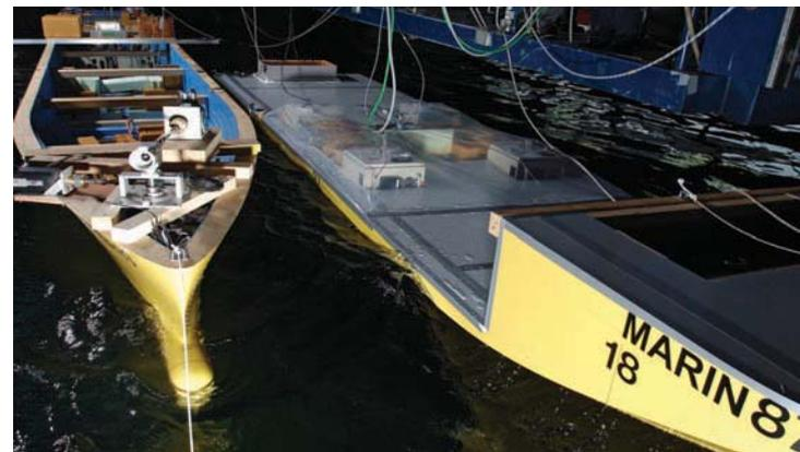
Figure 2: Example of ships operating side-by-side at forward speed at relative DP (STLVAST project). The model size is between 6 and 10 meter.
