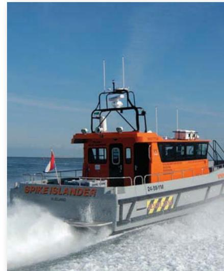
Ultra Dynamics supplied three sets of twin UltraJet UJ377 Waterjet installations to South Boats for their New Mk II GRP 43/12m WFSV RRV Catamarans RRV Audrey, Offshore Response 1, and Spike Islander. The GRP catamarans have all been tailored to meet specific code and operational requirements of Wind Farm operations operators Turbine Transfers (Holyhead Towing) and Offshore Wind Power Marine Services: Limited (OWPMS) and Waddentaxi in the Netherlands respectively.
