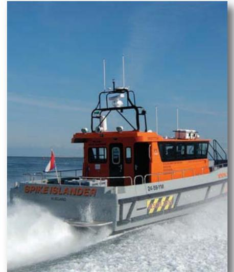
Ultra Dynamics supplied three sets of twin UltraJet UJ377 Waterjet installations to South Boats for their New Mk II GRP 43/12m WFSV RRV Catamarans RRV Audrey, Offshore Response 1, and Spike Islander. The GRP catamarans have all been tailored to meet specific code and operational requirements of Wind Farm operations operators Turbine Transfers (Holyhead Towing) and Offshore Wind Power Marine Services: Limited (OWPMS) and Waddentaxi in the Netherlands respectively.
