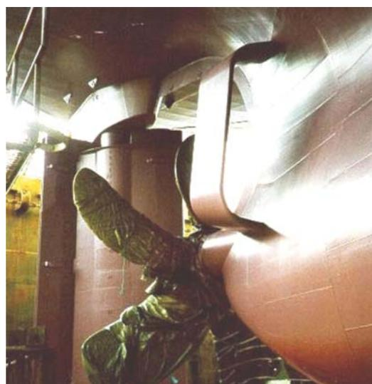
**Typical Stern-Appended Hydrodynamic Energy Saving Devices (ESD) applicable for single-screw, high block coefficient ships such as tankers and bulkers. (The first photo is a Propeller Cap Turbine (PCT) retro-fitted on a tanker which had been constructed with a Wake Equalizing Duct (WED). The second photo shows a chemical carrier under construction with the Simplified Compensative Nozzle (SCN) being installed.)**
