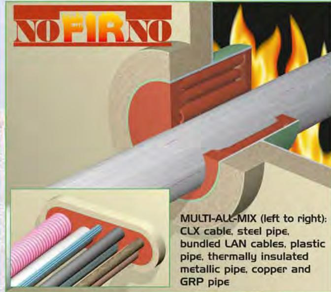
MULTI-ALL-MIX (left to right): CLX cable, steel pipe, bundled LAN cables, plastic pipe, thermally insulated metallic pipe, copper and GRP pipe
