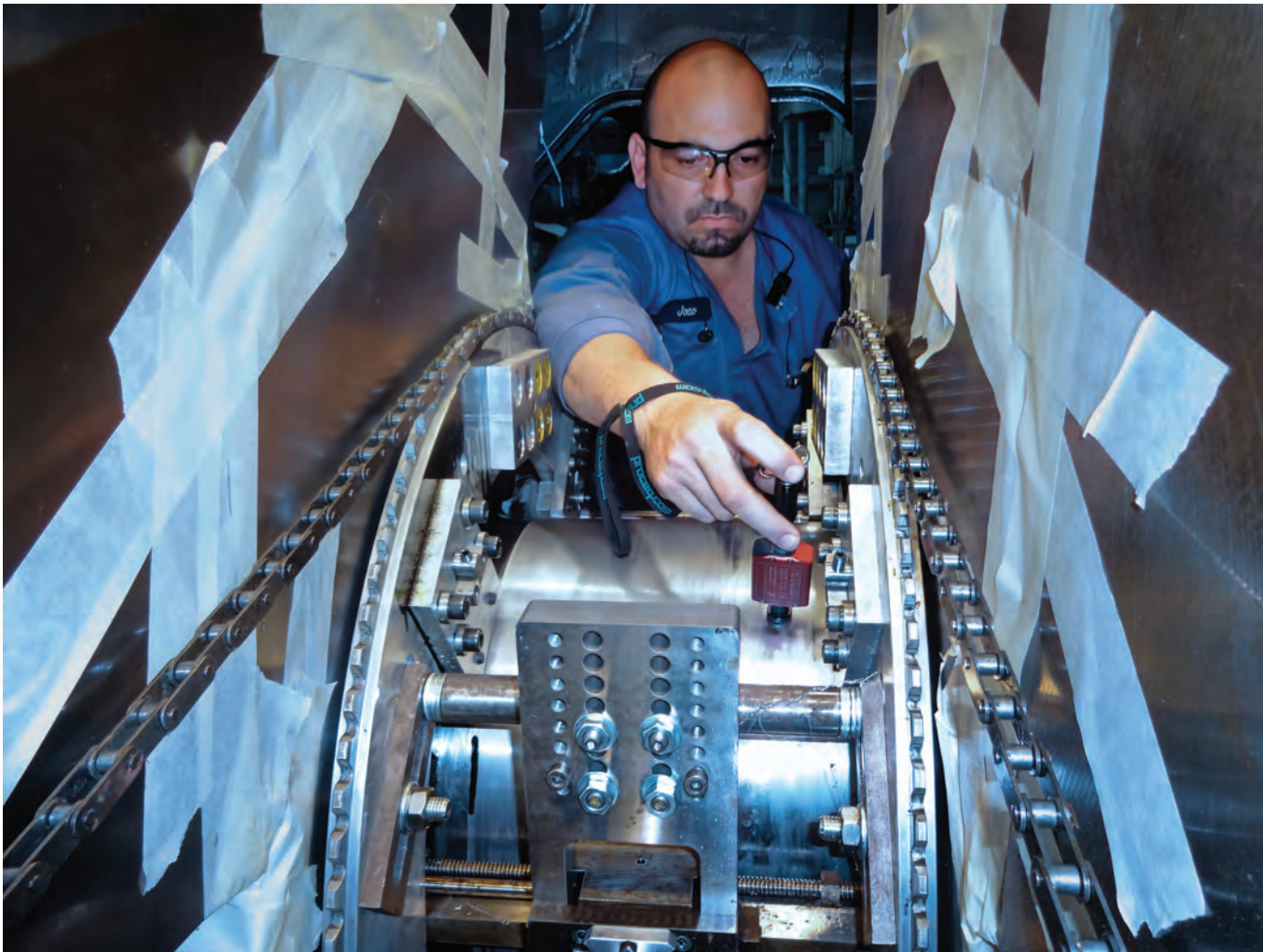
Golten In-Situ specialist checking journal hardness on a Pielstick 10PC2.4V main engine during crankshaft machining prior to annealing.
