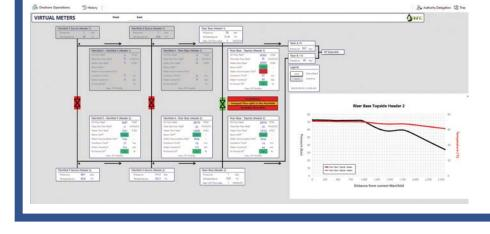
form. "It tells you you have 12 hours before you could begin to see hydrate risk based on current operating conditions, and here are your options, like injecting methanol at localized water accumulation spots or performing hot oil circulation or preparing for a blowdown," he says. And potential flow assurance problems can manifest a host of symptoms. Figuring those symptoms out requires "playing detective," Dinata says.
