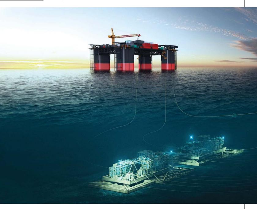
manned wellhead platforms or unmanned production platforms (UWP/UPP). These concepts, working remotely and unmanned, have the potential to save 30% capex and 50% in opex, according to an Equinor presentation from 2018.
