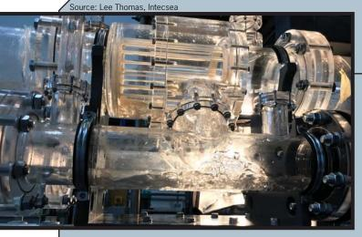
**PDG Unit in Testing:** A scale model test of the pseudo dry gas system has been put through its paces.
