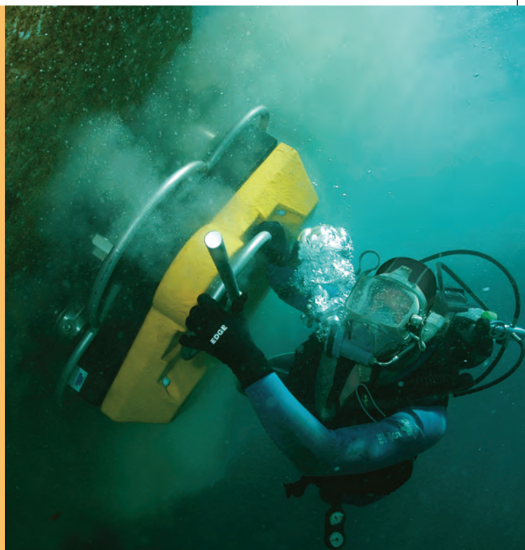
Diver cleaning biofouling
