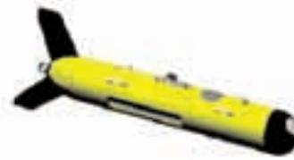
the offshore environment in mind. The C3D represents the latest in sonar technology with patented technology that incorporates a multi-array transducer and solving for multiple angles of arrival for a 3-dimensional image.
