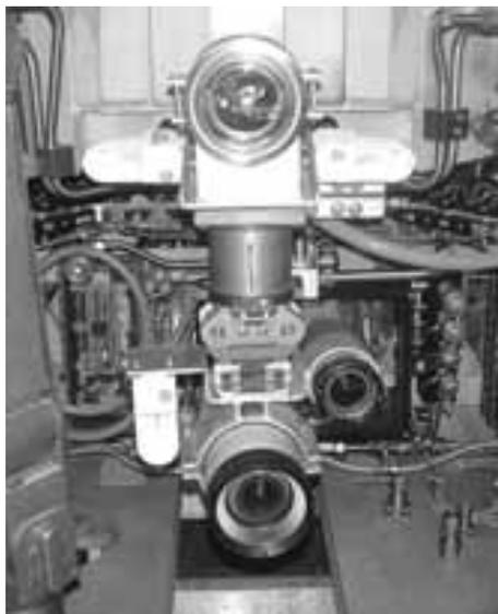
Lights, camera, action. This ROV carries several cameras and lights so the operator gets a clear picture of the work being done. Two work arms are at opposite sides of the photo.
