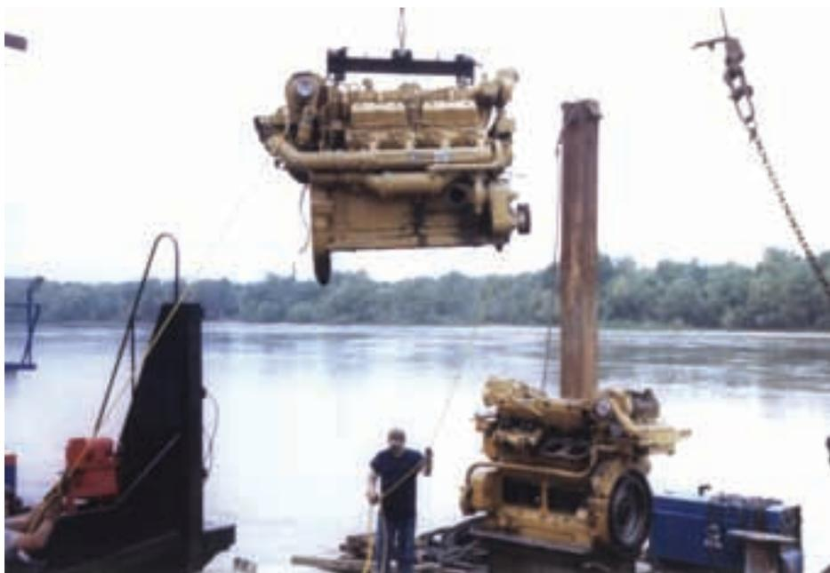
The M/V Sprig repower crew removes the original Cat D379 engines from the tugboat.
