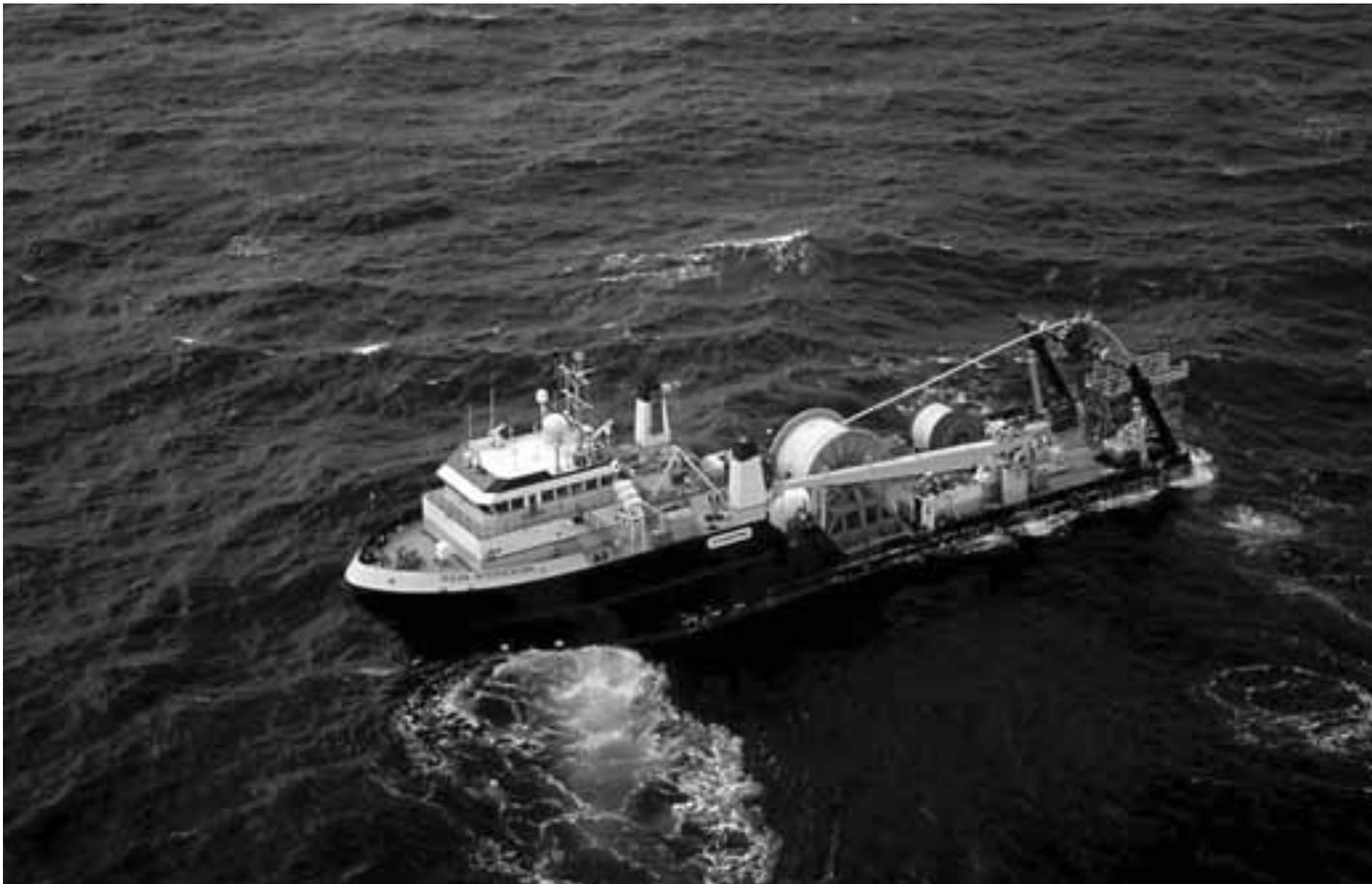
The Ocean Intervention, a very capable ROV support vessel with two moon pools, a heavy duty ROV, DP2 system and a 6,000 sq. ft rear deck.
