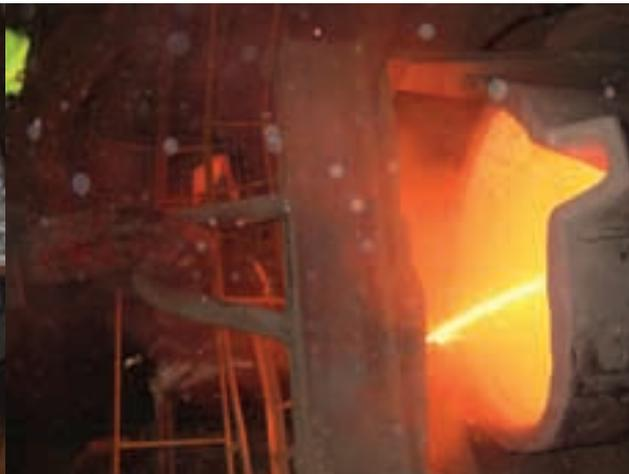
The liquefied metal literally runs out of the furnace and into a ladle to be transported to the mold.
