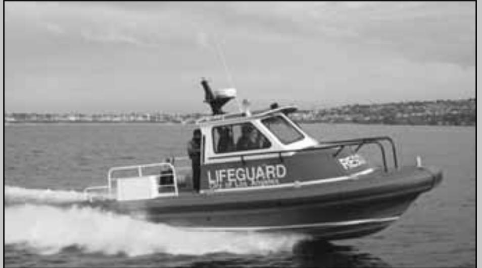
And, the pontoons are integrated into the hull, making entering, exiting and mooring the boat much easier than with conventional RIBs. As with the standard S-24 and the S-24SUN open bow, the S-24RIB boasts top-notch Gaffrig Platinum and Faria instruments and controls. The deck features all stainless pop-up cleats, handrails and pop-up lantern. Hydrolift has accommodated the crew and passengers with a host of interior amenities,
