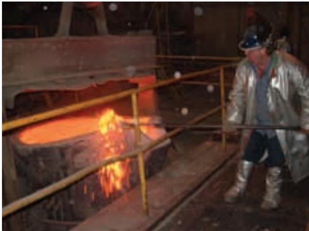
A worker in a fire resistant safety suit draws off a sample of the metal that is taken to an in-house lab for analysis.
