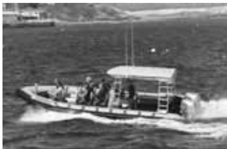
The Ribcraft 6.5 (21 ft.) was introduced this winter. Measuring over 21 ft., this RIB features Ribcraft's signature deep V hull design with full length lifting strakes and integrated internal stringer system as well as Ribcraft's multi chambered Hypalon tubes. Designed with all weather
