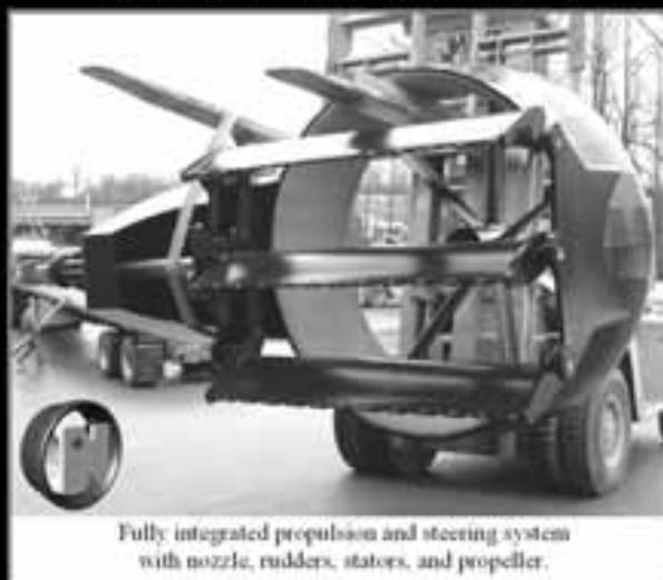
Fully integrated propulsion and steering system with nozzle, rudders, stators, and propeller.
