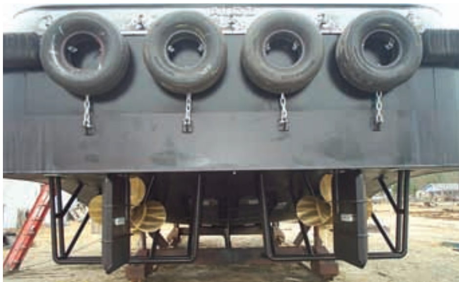
Rope guards to protect props and shaft
