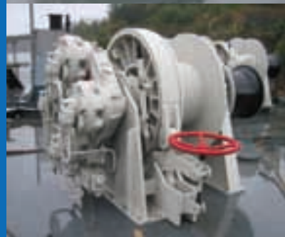
RESEARCH & SPECIALITY WINCHES -- This hydrographic is but one of several types aboard NOAA's FRV-40 Oscar Dyson
