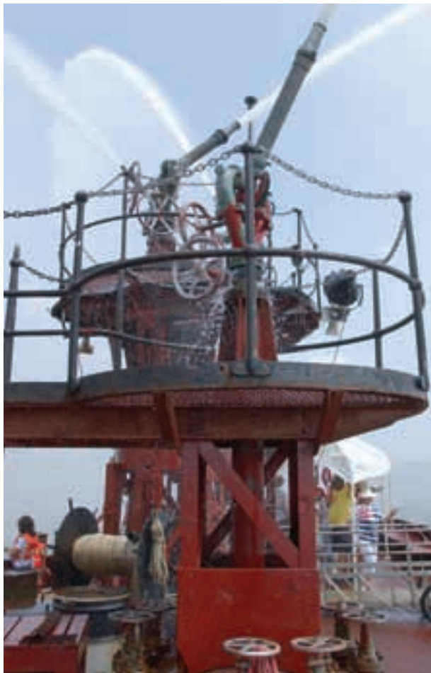
The John J. Harvey brought a lot of grief to a lot of fires in the years since 1931, its 18,000 GPM pouring through eight monitors and hose connects like these. (Photo: Don Sutherland.)
