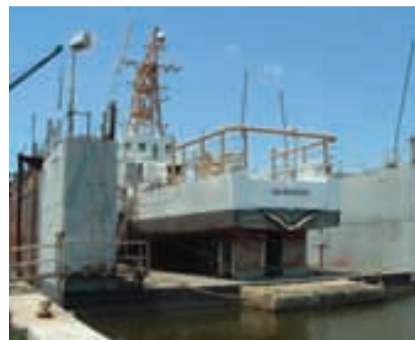
The 123-foot lengthened and modernized Vashon at Master Marine. The deep V notch in the stern of the Vashon is an obvious sign it is one of the renovated vessels. The V notch lifts up so a RIB can be self-deployed and recovered.
