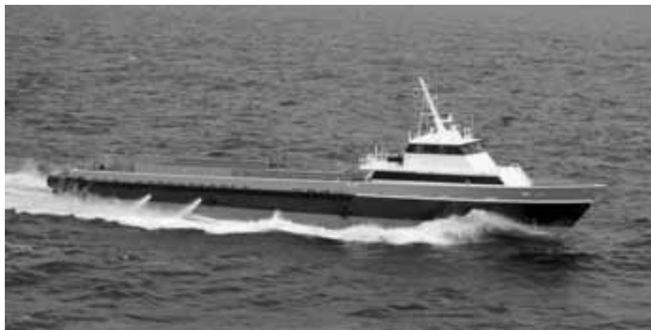
The 167-foot Mr. J.O. is an example of the application of Cummins engines. A quartet of KT-50's, with Tier One emissions, propels this crew/supply boat while a pair of 6BT engines, rated at Tier Two drive generators. The Mr. J.O. was built by Neauville Boat Works, Loreauville, La.
