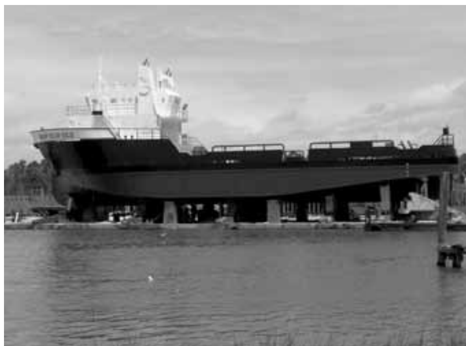
The Bishop Oscar Solis ready to be launched at Master Boat Builders, Bayou LaBatre, La. This 145-ft. supply boat for Abdon Callais Offshore is powered by a pair of Caterpillar 3508 engines, rated at Tier One. The auxiliary engines for electrical power are C-9, Tier Two engines.
