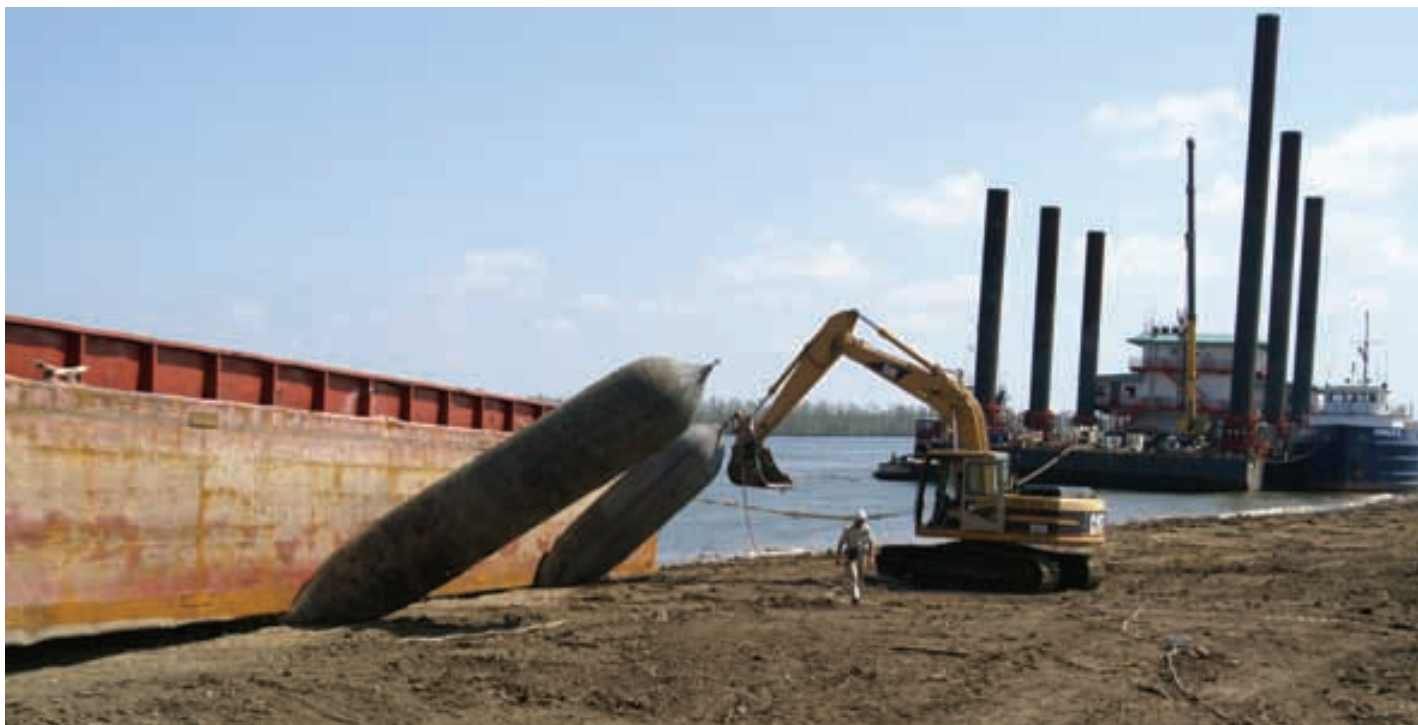
Near the 50-mile marker on the Mississippi, Titan Maritime uses inflatable airbags to lift one edge of a massive hopper barge off the levee, whereupon gravity helps return the vessel to the water. (Photo: Don Sutherland.)
