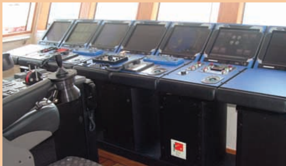
The newer 280-ft. vessels have a completely redesigned pilothouse with monitors replacing the various switches, dials and levers that populate most wheelhouses.
