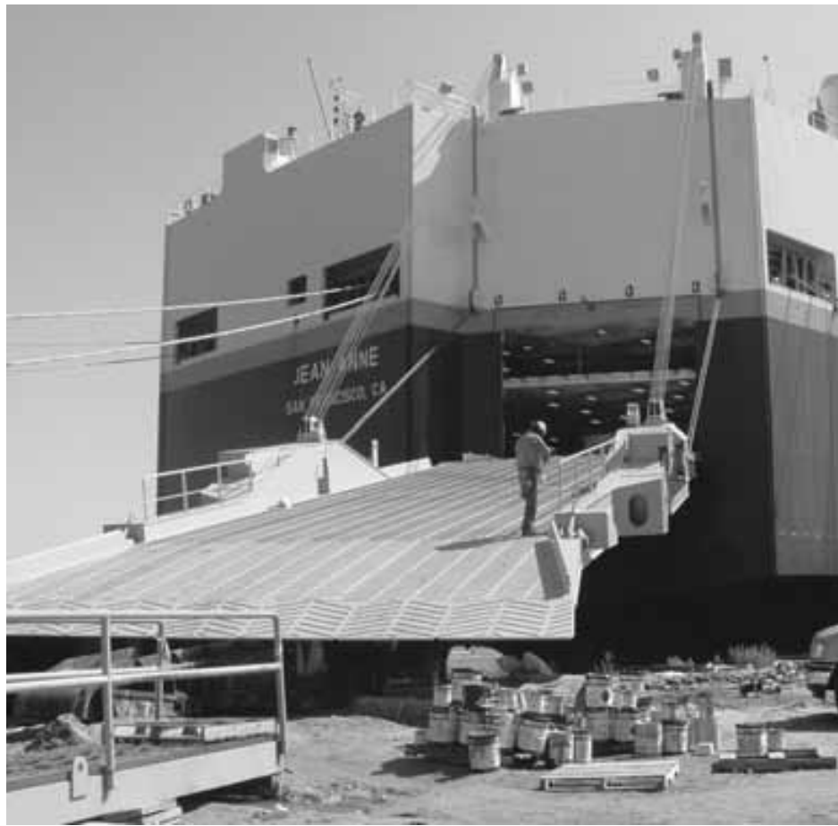
The 100-ton capacity of the aft ramp of the Jean Anne is used to load Over High and Wide vehicles such as buses, trucks and military vessels
