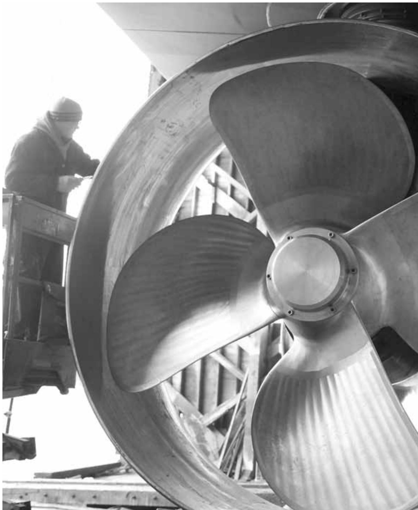
It takes a big propeller to move a tug against an LNG tanker underway. The pair on the Edward J. Moran are attached to Rolls Royce US 255 Z-drives, driven by two EMD 12-710-G7B main engines, bollard pull given as 176,760 lbs. ahead, 170,000 astern. (Photo: Don Sutherland.)
