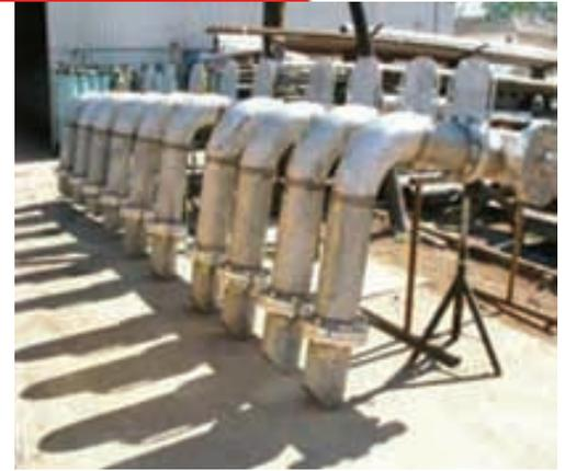
FABRICATION OF STAINLESS STEEL MANIFOLD
