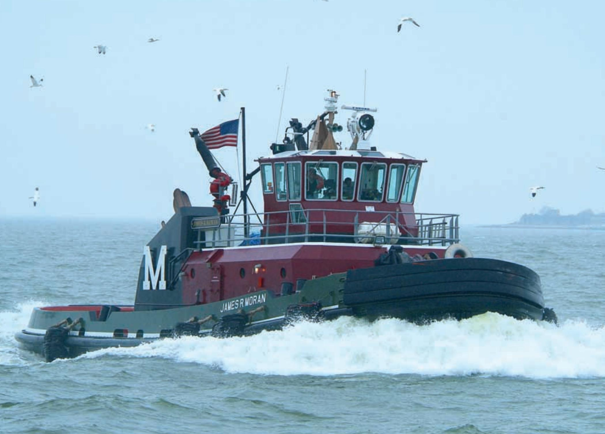
**James R. Moran, W&D hull 81, approaching Norfolk one year ago. A member of the Kaye class, the James has two EMD 12-645f7B main engines driving a pair of Ulstein 1650H Z-drives. Bollard pull ahead is given as 139,000 lbs; 135,000 astern. (Photo: Don Sutherland.)**
