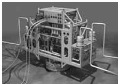
The MultiBooster subsea multi-phase pump system designed to deliver improved oil recovery and facilitates longer step-out distances between subsea assets and host facilities by lowering pressure at the reservoir and increasing pressure in the production line. Under development since 1998, the system utilizes twin-screw internals and Aker Kvaerner's pressure-volume regulator to provide a flexible and robust subsea solution.
