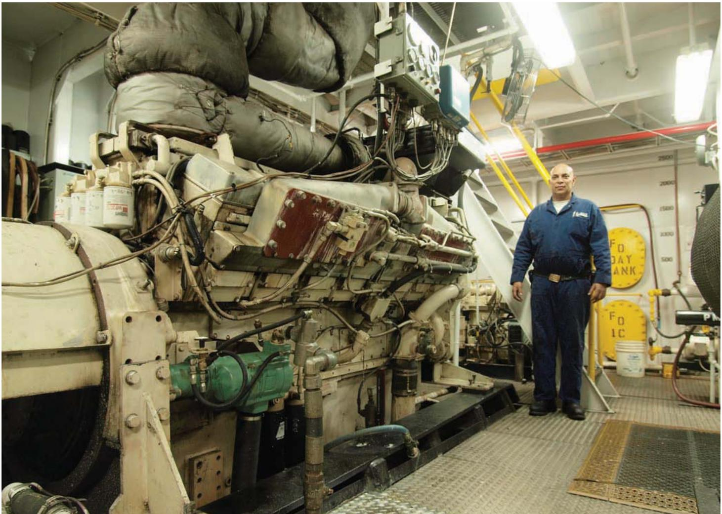
**Of the eight tugs built to the Emtech 100-ft design, only two — the Nathan E. Stewart and the Ross Sea — feature the compact Cummins KTA-50 16-cylinder engines. Ross Sea's engineer Lawrence Bethke respects the units, but said they're not as amenable to an engineer's teardown if required.**
