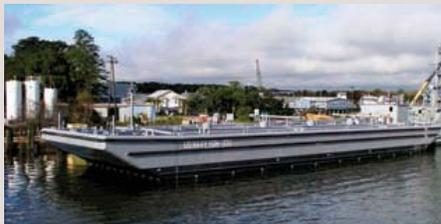
Metal Trades, Inc. announced the completion of YON 331, the second vessel of a new class of 14,000 barrel double hull fuel barges for the U.S. Navy. The 200-ft by 52-ft barge was designed by Bristol Harbor Group of Bristol, R.I. to carry either Diesel or JP5 Jet Fuel in five cargo tanks. Metal Trades was contracted by Maybank Industries of Charleston, S.C.
