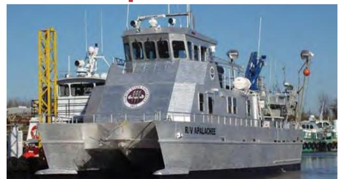
small ROV. The Apalachee structural design exceeds ABS high speed code for exposed routes and is USCG approved for 21 knots in 10 foot seas. The boat is outfitted with a custom 3000 pound capacity A-frame and trawl winch for over the stern operations. A Rapp Hydra Pro 5.5 mt knuckle boom crane on the port side is utilized for shore side transfer as well as offshore deployment of the Zodiac utility boat.
