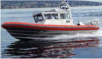
Kvichak Marine Industries, Inc. recently delivered the Patrol 28, a 28'x 9'3" all-aluminum vessel to the Boston Police Department Harbor Unit (BPD). Designed by Kvichak/Amgram Ltd., UK and built by Kvichak Marine, the Patrol 28 is effective for operation
