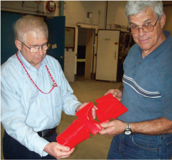
Chuck Ryerson and Len Zabilansky at the lab. They are holding a 3-D printed test article for understanding the effects of frazil ice in a water jet propulsion system.
