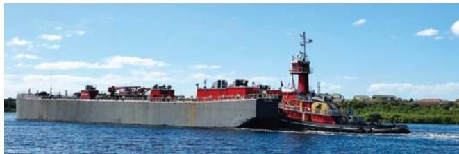
Bouchard Transportation Co., Inc. announced that Bouchard Barge No. 295 has completed a major overhaul. Approximately 90% of the B. No. 295's main deck plate has been replaced, freshly painted and triple-coated. New internal coatings have been applied, along with the instal-
