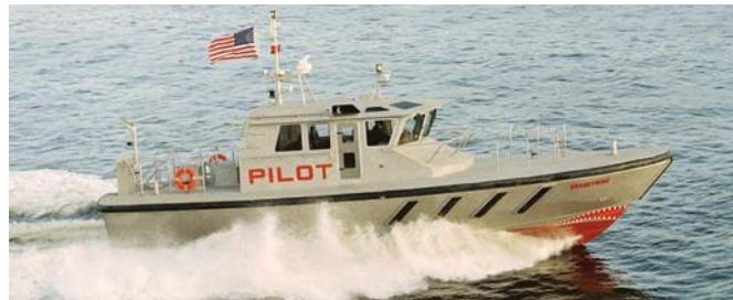
ter cooling to keel cooling, using Fernstrum grid coolers. A Humphree interceptor trim control system, with automatic trim control, was installed at the transom. The hull's fendering system was replaced with Duramax replacement rubber, along with additional diagonal strakes aft.
