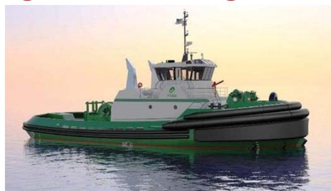
and a spacious engine room along with an anchor windlass and chain locker. The tugs will come with a 900 GPM fire pump and monitor and will be Subchapter M compliant.
