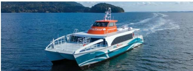
All American Marine, Inc. (AAM) has delivered the second of three low wake and high-speed passenger vessels for Kitsap Transit. The Reliance, an aluminum catamaran with a composite superstructure, was launched in Bellingham on March 6, 2019 and has been undergoing sea trials and wake-wash testing this past month. During these test
