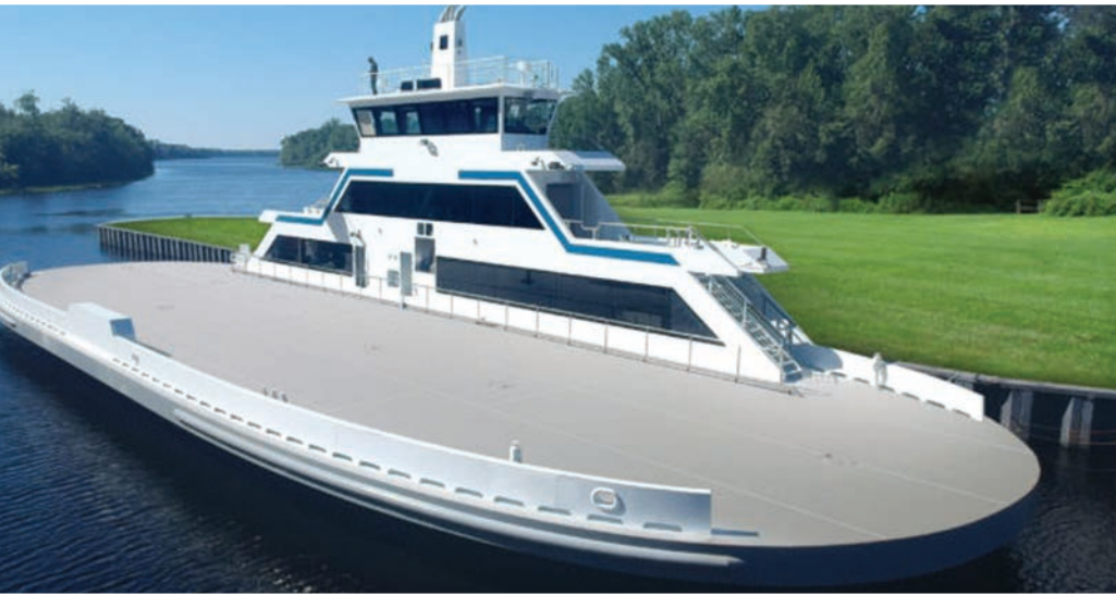
The second of four new 152'x 52'x 12', 150-passenger, 30-vehicle ferries, designed by Seattle-based Elliott Bay Design Group.
