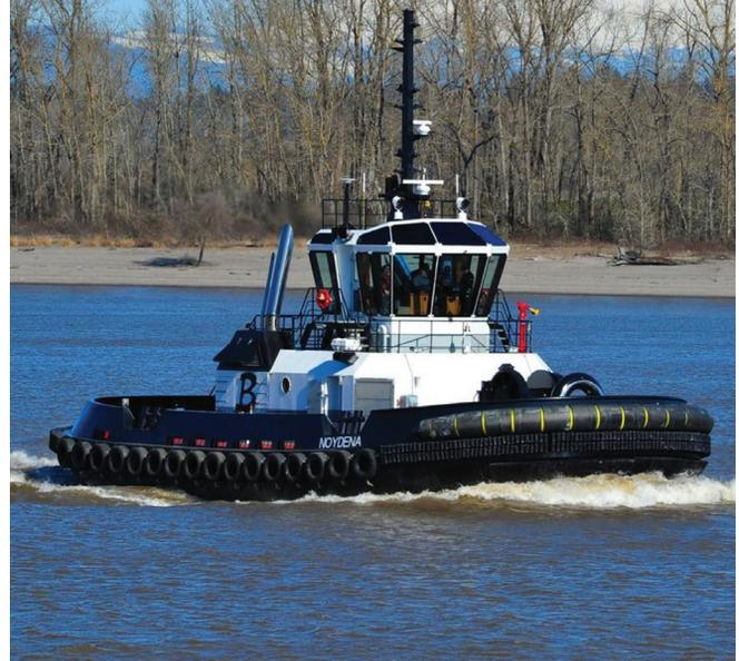
**Earl W Redd, built by Diversified Marine, Inc for Tug Construction in 2017, was the United States’ first EPA Tier 4 workboat. Foss Maritime is currently operating the vessel under bareboat charter for the U.S. offshore wind industry.**
