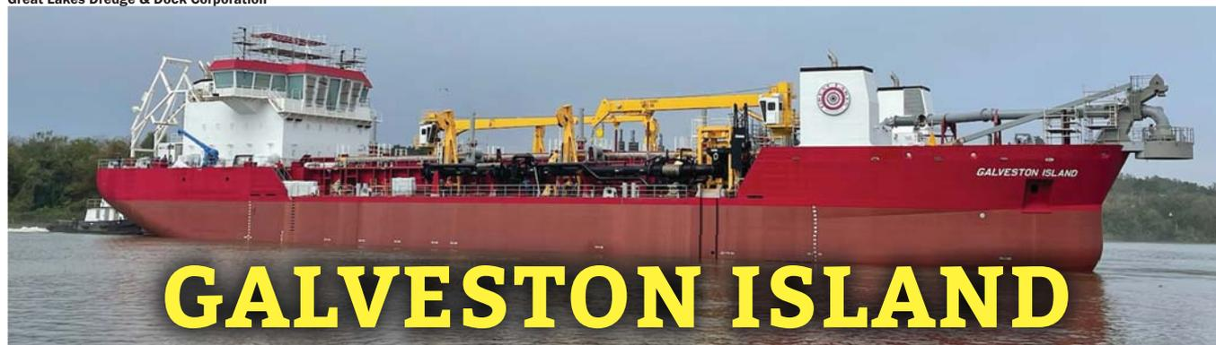
Delivered this year amid an ongoing dredge building boom in the United States, Galveston Island is the first in a series of two new 6,500-cubic-yard-capacity trailing suction hopper dredges (TSHD) designed by C-Job and constructed by Conrad Shipyard for Great Lakes Dredge & Dock Corporation as part of the Houston-based dredging contractor's fleet renewal program.
