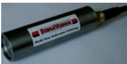
Sonavision Limited's new model for the Hawkeye range of video cameras is the Hawkeye 65CT, designed as a lightweight titanium-housed color camera, with an electronics balanced line driver capable of delivering video over a 500 m twisted pair cable, or via a 1,000 m coaxial cable. Designed for use by commercial divers over long umbilicals, the camera weighs 150 g, is 140 mm long and 36 mm in diameter.
