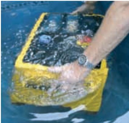
A new, completely sealed and waterproof surface control unit for ROV operations has been developed by Seaeye. The unit is rated to the international standard IP68, and is designed to withstand emersion to one meter. Designed for use with their Seaeye Falcon ROV, the unit's special sealing arrangements and slipping hinge between base and lid, means it is also fully protected against dust ingress in any hazardous shore-based environment.
