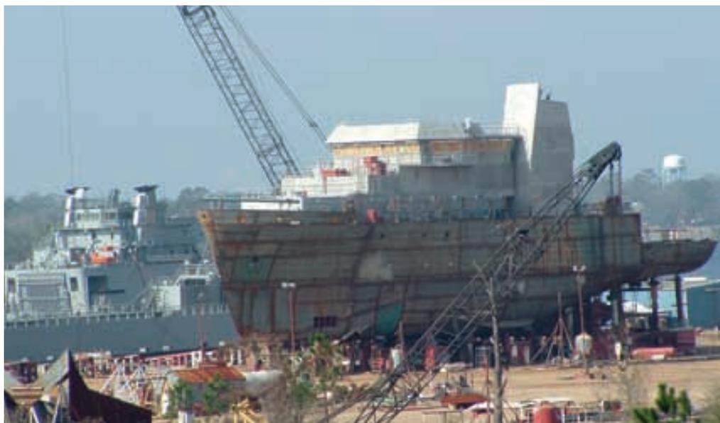
Henry B. Bigelow under construction on land at a VT Halter shipyard.
