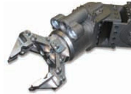
Schilling Robotics' new integrated wrist camera for TITAN manipulators features a titanium camera housing for protection and internal cabling that is designed to eliminate cable snags and abrasions. The high-resolution color camera, which includes LED lights with two illumination levels, can be ordered in either NTSC or PAL format. The depth rating is 4000 m.
