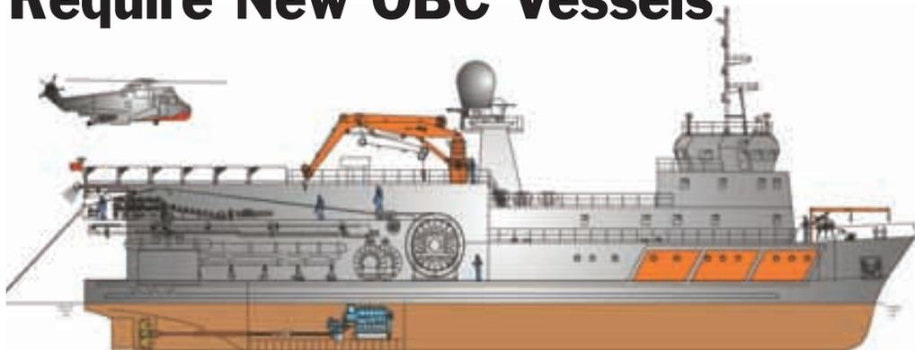
Complete twin-screw medium speed propulsion packages have been ordered from MAN B&W for a twin set of 65 m off-shore research vessels. The twins will each be specified and equipped for specific operational tasks, i.e. seismic sourcing and seismic recording. The vessels are designated as an OBC Source Vessel and an OBC (Ocean Bottom Cable) Recorder Vessel, respectively.
