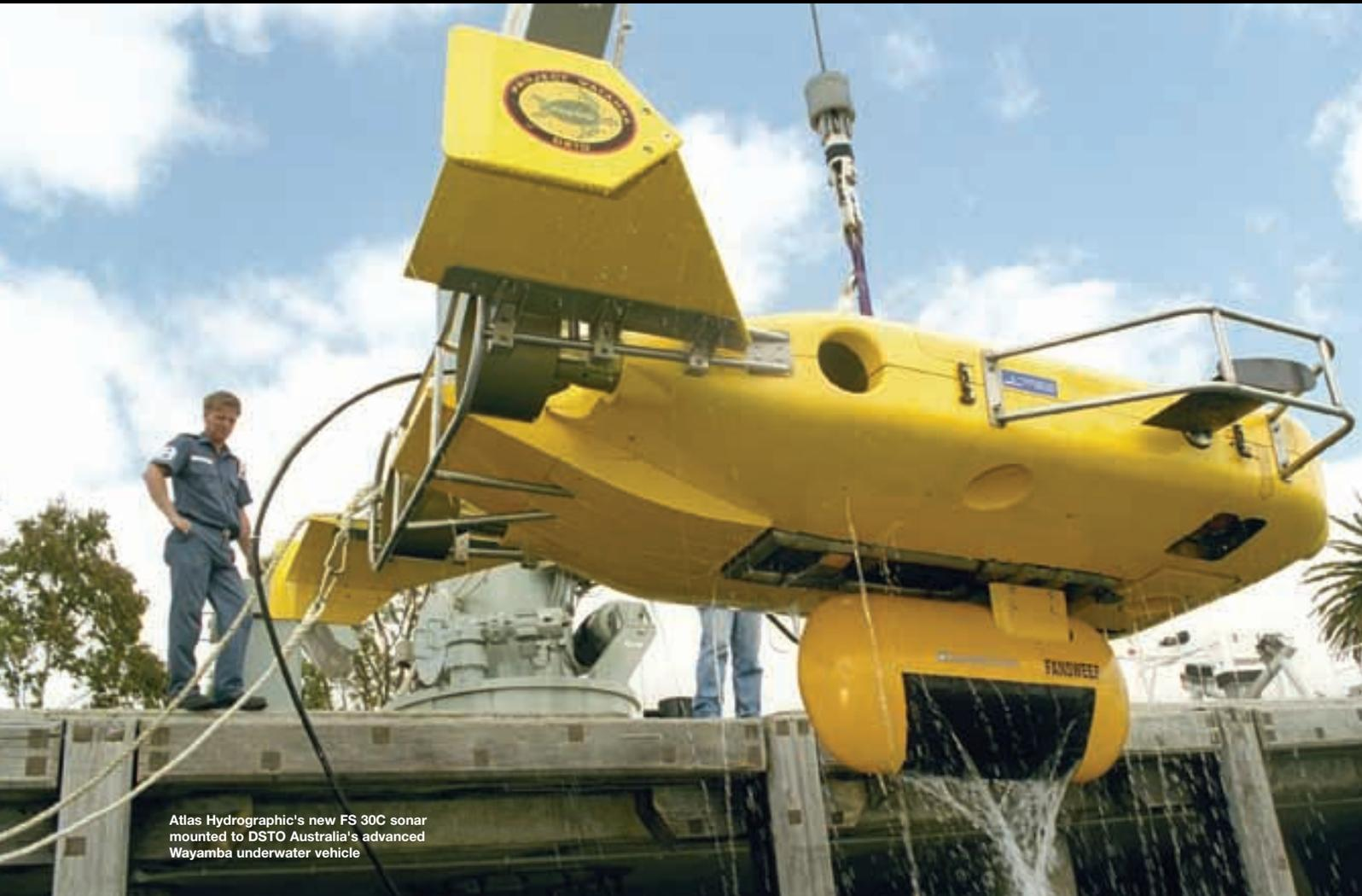
Atlas Hydrographic's new FS 30C sonar mounted to DSTO Australia's advanced Wayamba underwater vehicle
