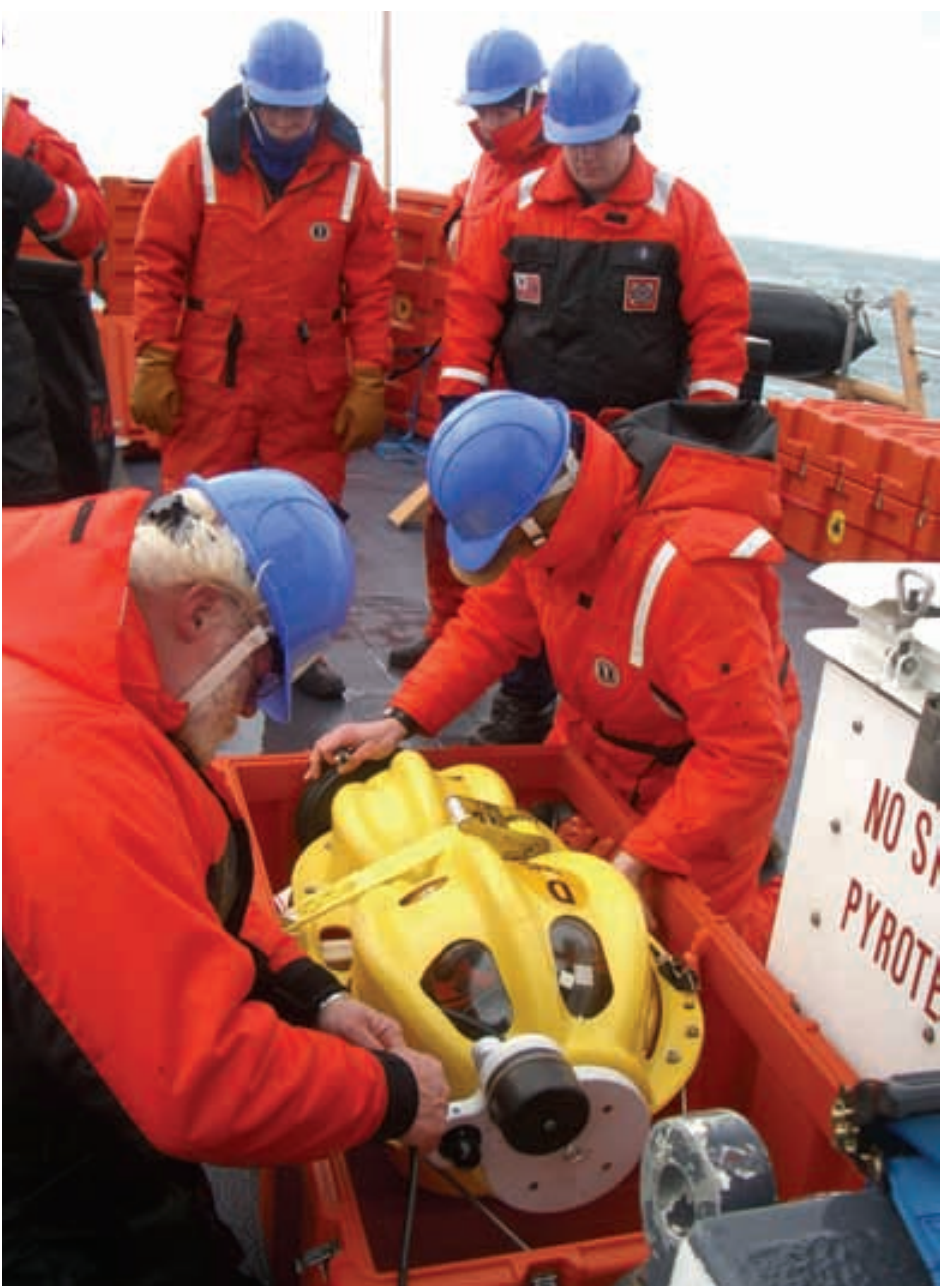
Science team members, assisted by cutter Roanoke Island's crew, ready an OBS to be hooked to the crane, hoisted over the side and dropped to the ocean floor. (Photo courtesy of U.S. Coast Guard cutter Roanoke Island.)
