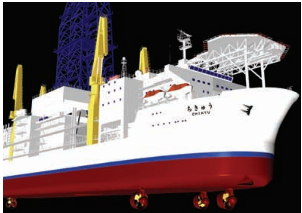
Thrusters (propellers) on the hull CAD computer model. (Photo credit: JAMSTEC)
