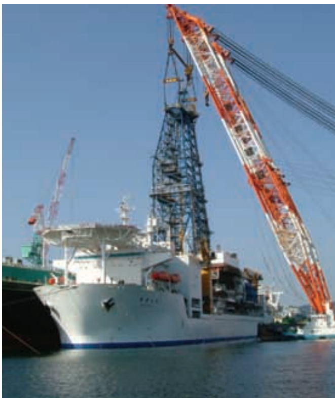
The derrick has just been installed. (Photo credit: JAMSTEC)
