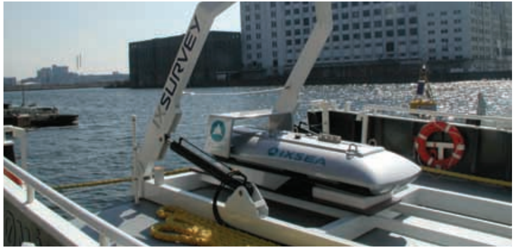
The new IXSEA Synthetic Aperture Sonar Towed fish aboard the new IXSURVEY vessel.
