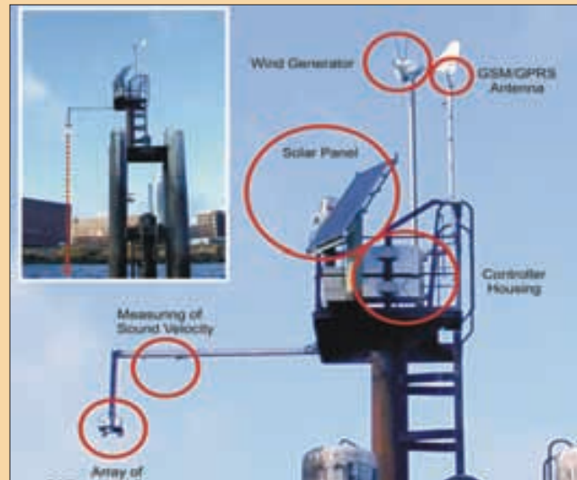
The Tide and Wave Station LOG_aLevel winner of Rijkswaterstaats' comparison test 2005.
