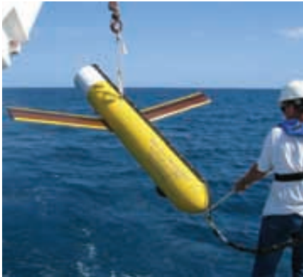
Edge Tech's latest technology - Buried Object Scanning Sonar (BOSS) System - which is currently under development with Florida Atlantic University for the U.S. Navy.
