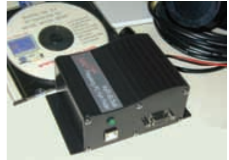
The PcFF80 is a dual frequency PC based sonar costing less than $1,000, including the transducer and software for WinXp, Win2K and Win98.
