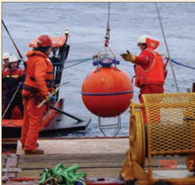
Thales Geosolutions 75 kHz RDI WH ADCP in Flotec Buoy.
