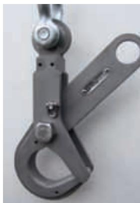
McMillan Design, Inc. introduced the Sea Catch Off-Load Hook OLH25 designed to safely lower a load to the seabed and automatically release the load upon reaching the seabed. The flexibility of using common shackles as a counterweight, generous capacity, and a lighter unit weight are a few of many features that make this off-load hook unique.
