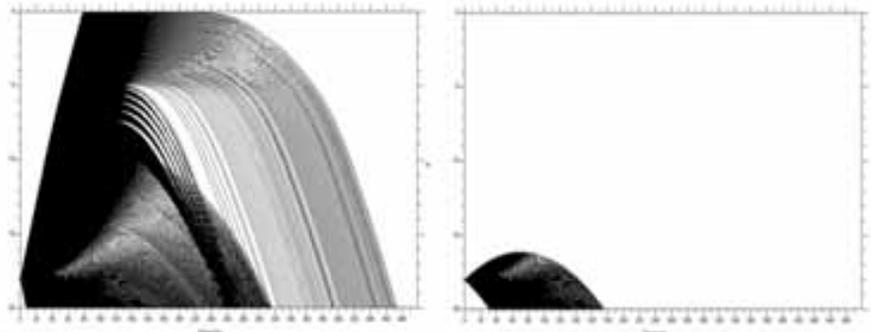
**Raytrace for Downward Refracting Sound Speed Profile for Cerberus Vertical Field of View (left hand side) and narrow field of view sonar (right hand side).**
