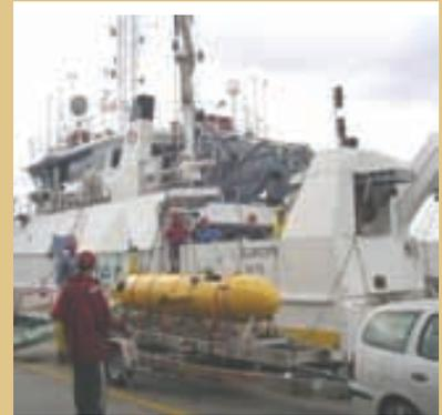
proven it's capabilities for the operational oceanographic service." IFREMER took its first Explorer AUV in 2004. This latest delivery is the fourth of the class, and a fifth is currently in production for the University of Bremen, Germany. The Explorer vehicle was designed to operate from small vessels of opportunity, and has a level of modularity that allows it to be fitted with a wide variety of payload instrumentation.
