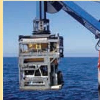
The Seaeye Cougar system is shown being recovered following operations to lift and relay an acoustic tracking range at depths of over 1,500 m.
