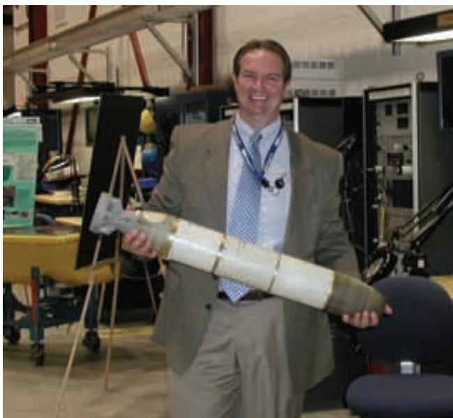
**NUWC's Jim Spessor holding the Lockheed Martin EMATT Submarine Target Practice AUV, the smallest of the UUV fleet.** (Photo Credit: Maggie L. Merrill, MTR)
