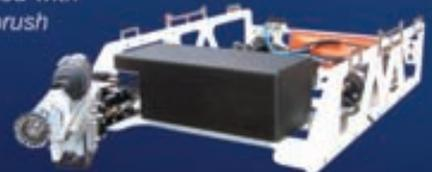
*Manipulator with water jet and disc cutter on extender*
