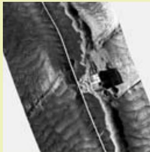
Additionally, representatives at Noordhoek had the following to say: "The data recorded was quite simply excellent, proven by the sample below. The pipeline entering the protective structure is seen quite clearly and even the gaps between the mattresses covering the pipeline on the port channel are displayed." EdgeTech can provide systems for most ROTVs as well as engineered to order systems for custom marine applications where gathering of sonar data is required.
