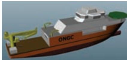
al regulations, International Association of Classification Society, Indian Registry of Shipping and Directorate of General Shipping certification. The vessel is to be equipped for high pressure pumping operations and storage facilities with various blends of chemicals including sand, flow back facility and burner boom, and will feature a helicopter deck and three cranes.
