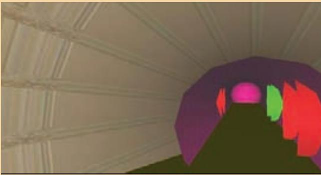
**A view from the perspective of the Falcon, from within the Shaft 1 chamber alongside the elevator that carried the deployment garage to the 480-meter level. SeaVision color-coded the different spurs off of the primary drift so that the SeaView's ROV operator knew which tunnel was the target. The spur tunnels do not actually come into the interior of the main drift; rather, that is an artifact of the 3DTV shapes used to develop the concept model for the project.**
