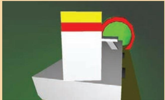
A view of the SeaEye Falcon (yellow, red, and white rectangular prism) navigating within the 3-D conceptual model of the tunnel. The object under the ROV is a concept of a scoop loader, which had been abandoned directly adjacent to the narrowed sidewalls that lead to the bulkhead door (marked in the background as the red toroid). Note that the ROV is hovering above the scoop loader and that a roof over the scoop loader operator station may be either an obstacle or an entanglement hazard.
