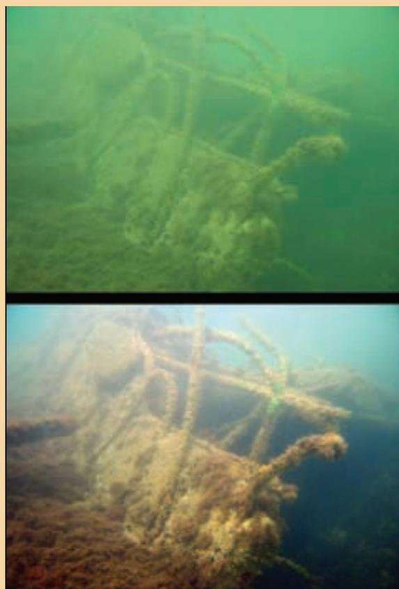
Visual enhancement technologies, such as those being developed by **LYYN AB**, help to improve visibility in turbid subsea environments. (Image from <http://www.lyyn.com>)
