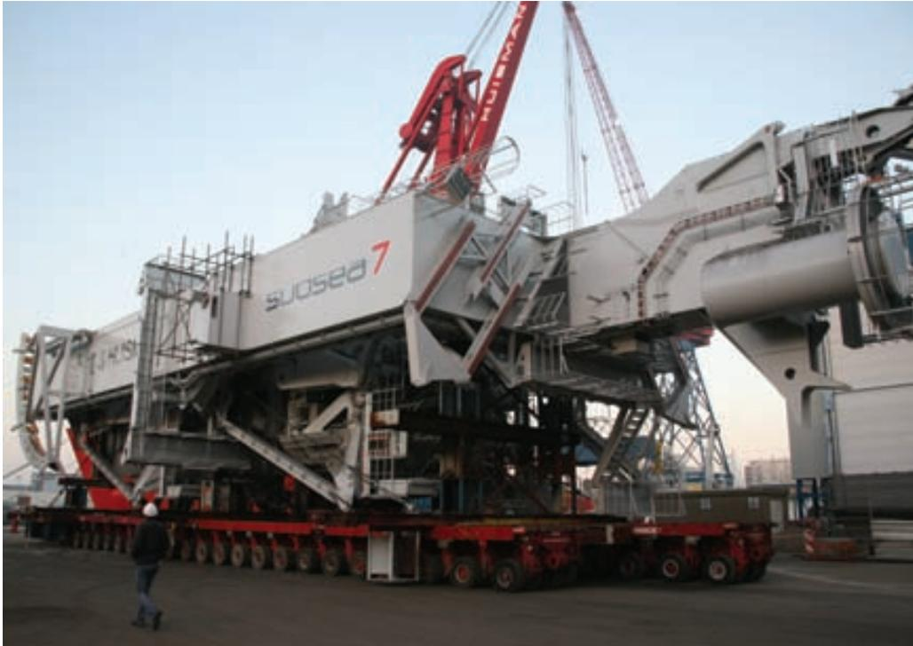
sioner, a retractable electric driven main tensioner (260 t flex rated, 400 t rigid rated) and an enclosed welding station for J-Lay operations. Two hold carousels with a storage capacity of 1250 t each are provided. A 450 t and a 125 t A+R winch are provided. The moonpool hatches have a capacity of 750 t SWL.
