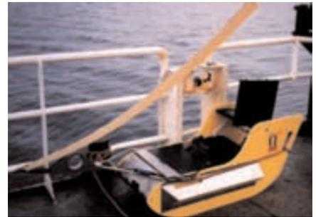
non-conducting cable. Its undulation instructions are preloaded into the built-in controller, which is powered by the vehicle's impeller driven alternator, which allow deployment from ordinary winches and capstans. Real-time flight control and data acquisition can be obtained via conducting cable.
