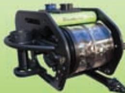
As a stand alone ROV or simply ROV mode the LBV150SE-5<sup>2</sup> is a highly capable free swimming ROV. Equipped with all the standard features of the proven LBV line of MiniROVs.
