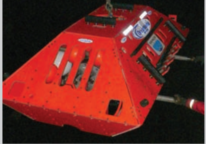
Cabled Observatory Node for the University of Victoria project VENUS as it is being launched.
