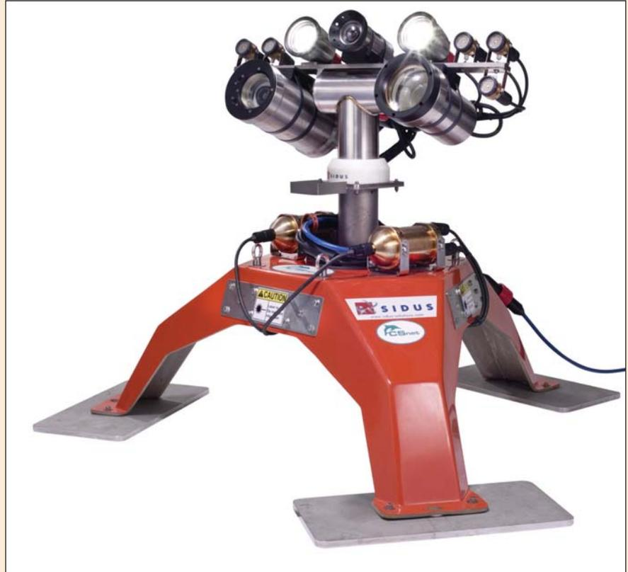
scaling lasers allows for image scaling and object distance measurement.
