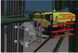
Range Ultrasonic Tool (LRUT) designed to be deployed by ROV and clamp around vertical or horizontal jacket tubulars. Fugro GRL created a simulation of the deployment of
