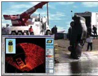
**Car being removed from canal; Inset photo – scanning sonar image of car on river bottom.**
