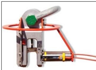
Martensitic Stainless steel 17/4PH The pin is standard shackle pin. The Imenco Shackle comes in various sizes 6.5T – 12T – 17T – 25T- 25T- 35T – 55T – 85T – 150Tons. Safety factor is 5. Any certification can be provided according to client's instruction.
