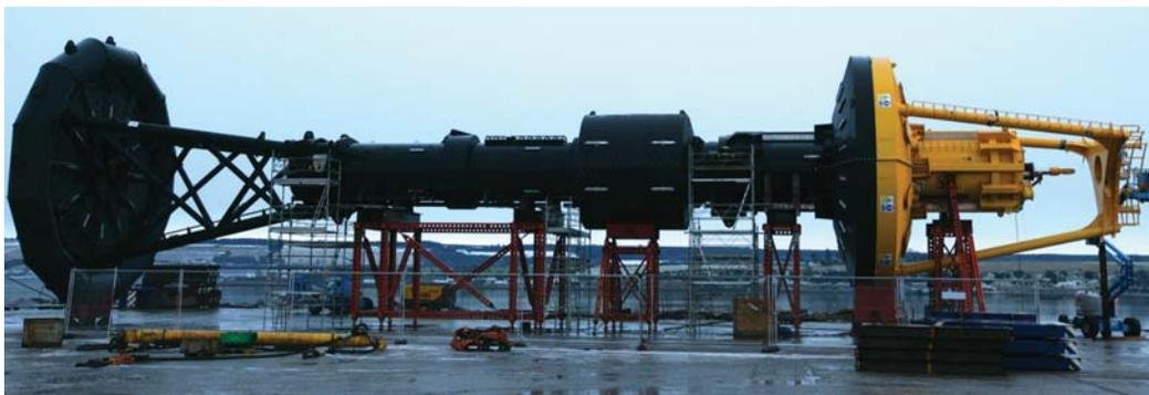
Ocean Power Technologies completed the first of its new generation utility-scale PowerBuoy device, the PB150. The PB150 PowerBuoy is touted by the maker as the largest and most powerful wave power device designed by OPT to date. With a peak-rated power output of 150 kW, the PB150 is designed for use in arrays for grid-connected power generation projects worldwide.
