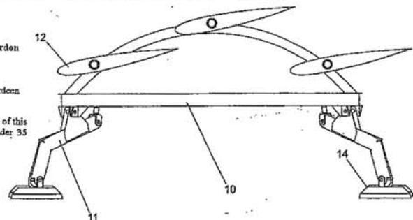
(Research cost £0.25 million; prototype could hold a 5m turbine in a 3m/sec flow, by friction only)
