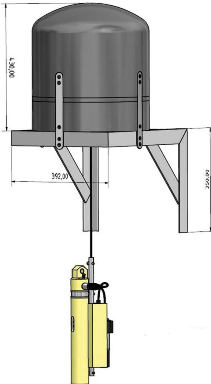
Profiling Control Unit APC506 with bracket.
