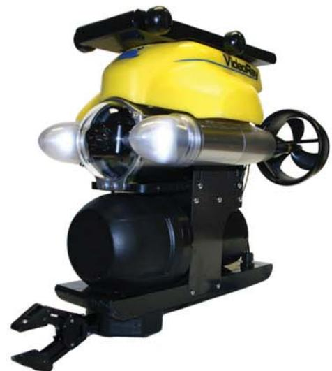
ABOVE: A Sheriff Diver deploys a VideoRay P4 Port Security ROV Configuration equipped with a hull crawler, high definition sonar, video enhancement, manipulator arm, and a GPS Smart Tether positioning system.
