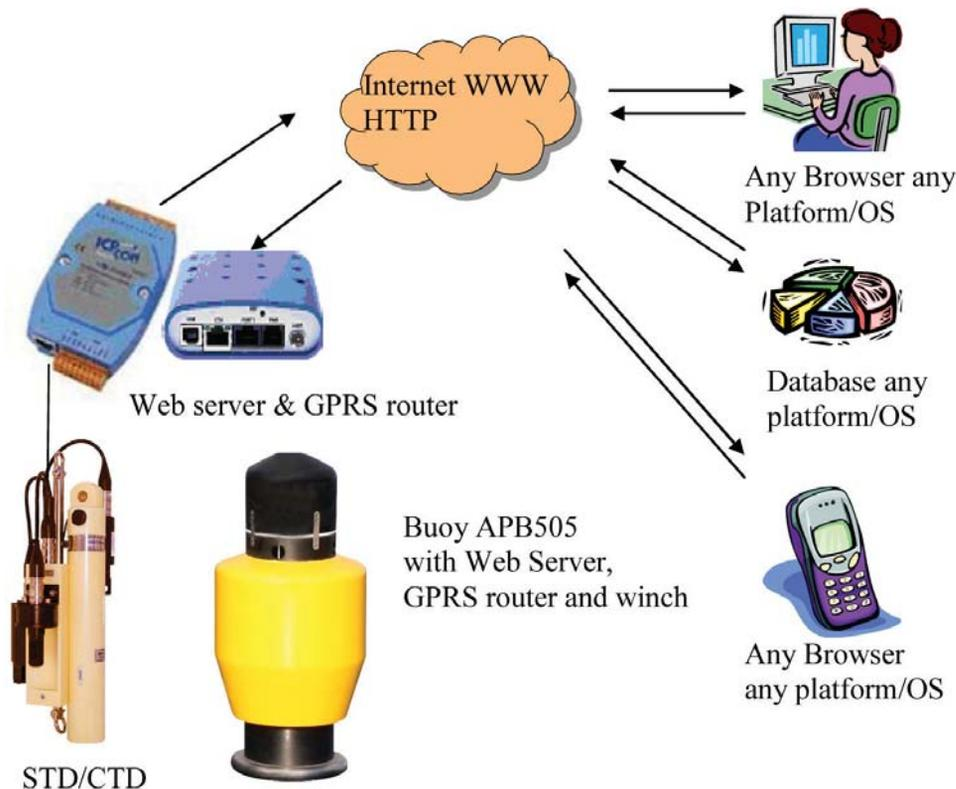
**Web server with dynamic HTTP using GPRS router to the WWW: Many users can connect at any time without interrupting measuring sequence at the platform.**
