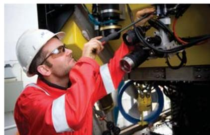
**James Rae, S3 ROV Pilot Technician, adjusting the camera pan and tilt unit on an S3 ROV.**
