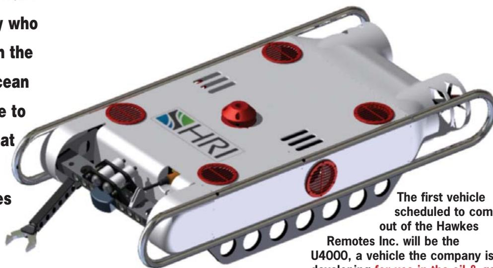
The first vehicle scheduled to come out of the Hawkes Remotes Inc. will be the U4000, a vehicle the company is developing for use in the oil & gas and environmental sciences field.
