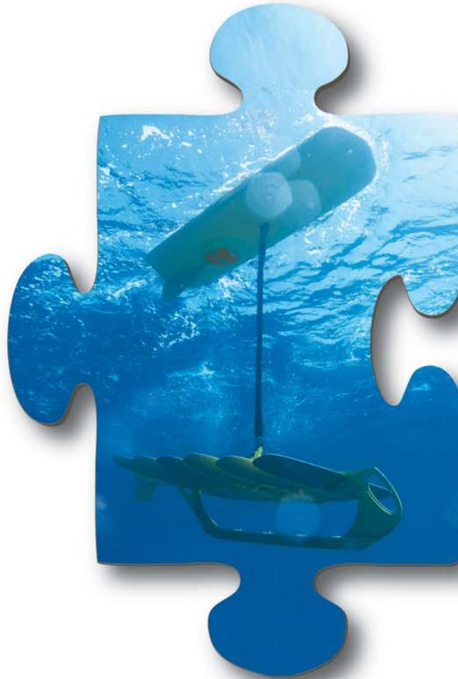
The **Wave Glider™** by Liquid Robotics is a versatile platform ready for subsea support. With proven meteorology and oceanography payloads you can monitor ocean conditions in near-real time. The Gateway configuration provides telemetry between fixed and mobile undersea nodes and operators ashore. Using innovative wave energy propulsion, persistent presence in the ocean is now available. Capitalize on this innovation to bring improved operational economics and safety to your operations today.
