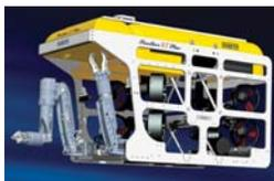
With 50% more power, and swimming 30% faster, operators value the ability of the new Panther to hold steady in strong shallow-water currents. Although rated to 1500m water depth, the application of the Panther XT Plus in high current shallow water locations is creating the main interest from customers who wish to have more capability in these more difficult areas of operation.
