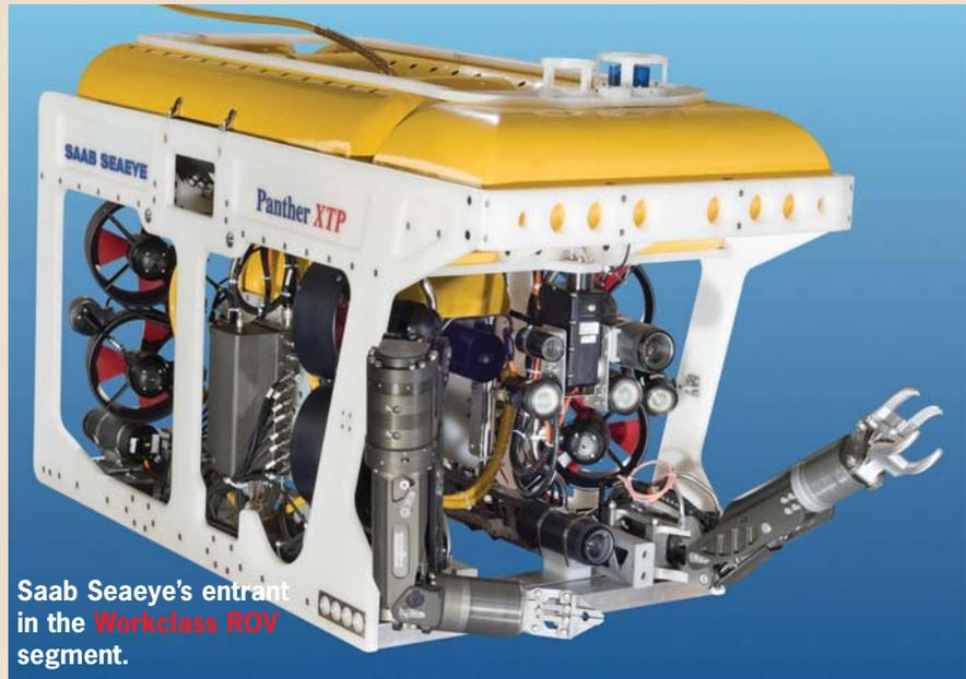
Saab Seaeeye's entrant in the Workclass ROV segment.
