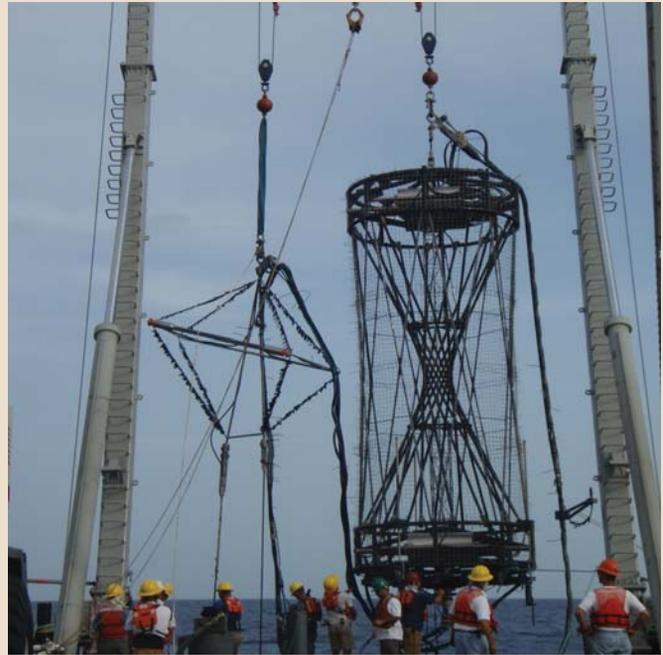
**SEAFAC/STAFAC HFA and HGMS Radiated Noise Measurement Arrays designed and built by CTG divisions Sonatech, ITC and Channel Industries.**
