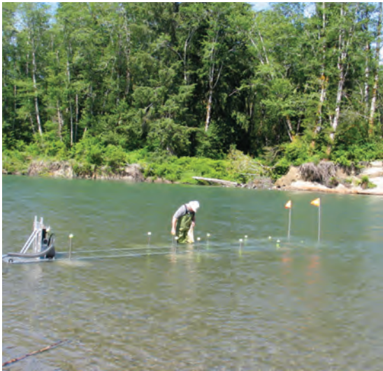
Installing the track (left) and the transducer (right).
