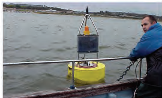
A pontoon buoy supports dual-depth water-quality instrumentation and power supplies for monitoring
