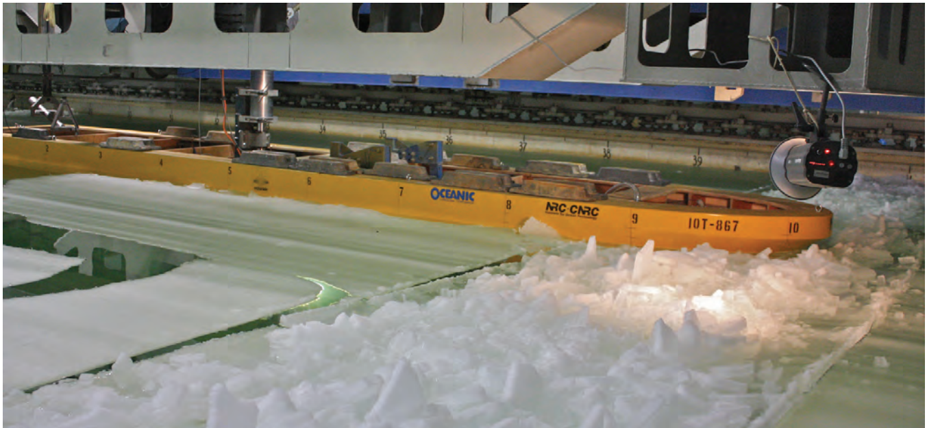
Oceanic Consulting Corporation research on ice loads on an FPSO from a first-year ice ridge, in the ice tank at NRC-IOT
