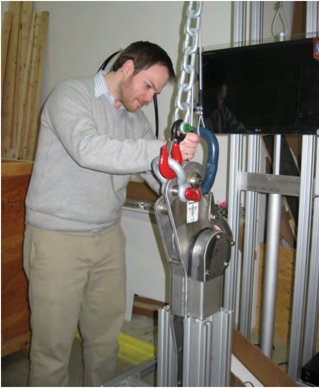
VMT Production Engineer Andrew Edwards explains the procedural hook trainer which teaches how to safely prepare lifeboat hooks for launch.
