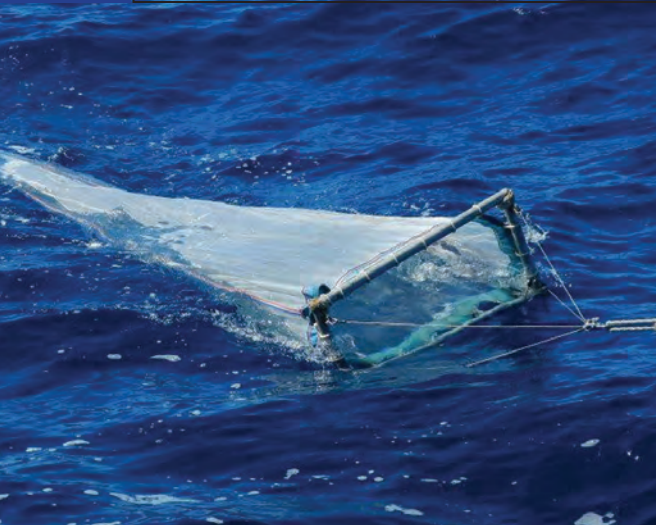
The neuston net sampling the surface of the ocean for plastic.
