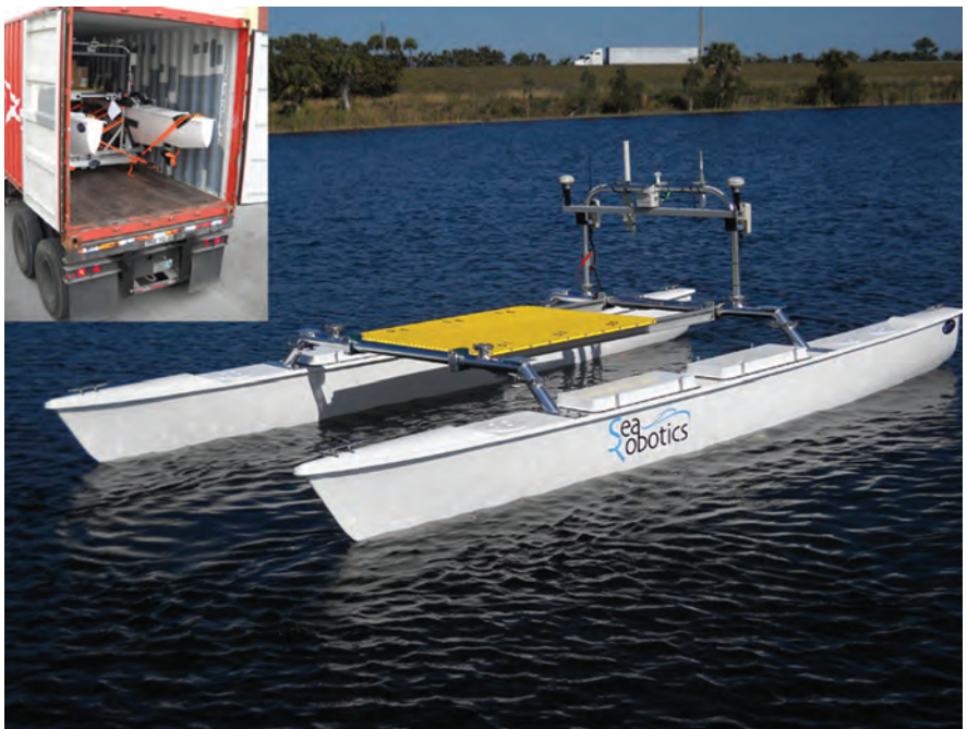
SeaRobotics' containerized 5.7-m USV to the NATO CMRE.
