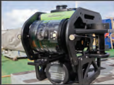
LBV300-5 - versatile dual vertical thruster ROV system.
