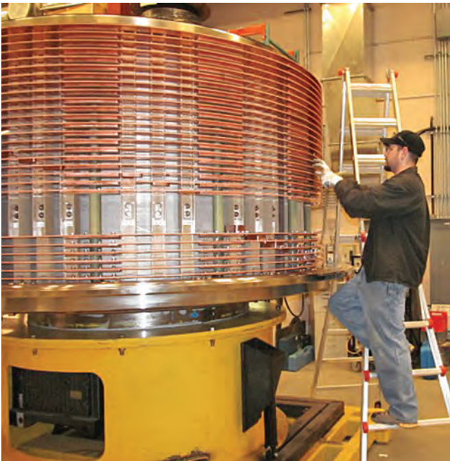
An employee works on the production of a large electrical slip ring at Moog Focal's Nova Scotia facility.
