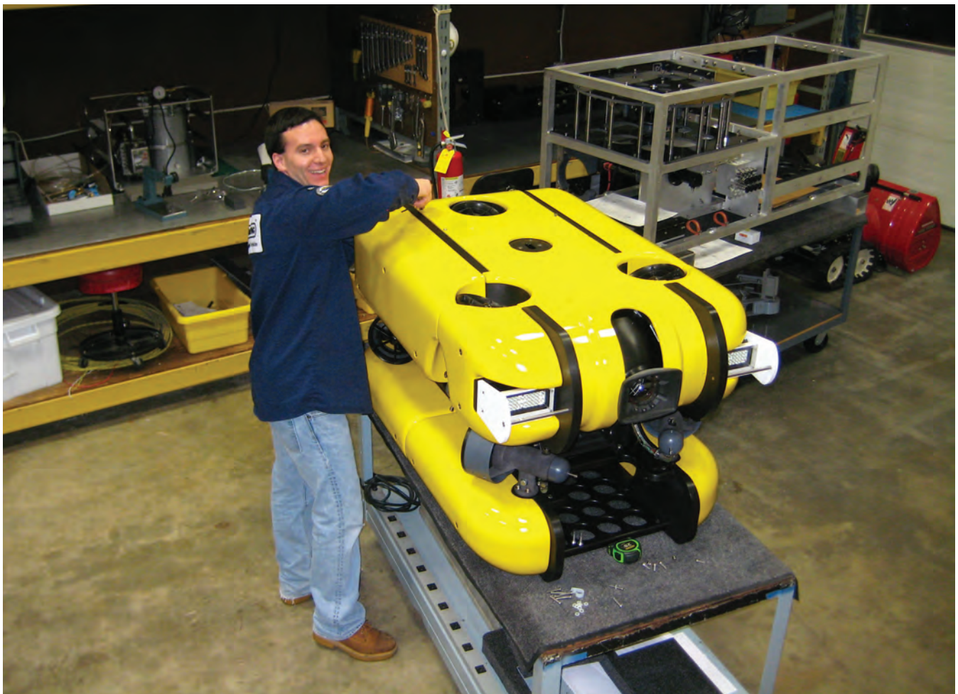
Below Oceaneering subsidiary Deep Sea Systems (DSSI) has designed and built the Sea Maxx Sat- ellite Remotely Operated Vehicle (SAT-ROV) to work in tandem with work class ROVs at depths up to 4,400m.
