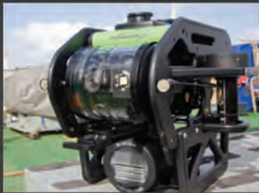
LBV300-5 - versatile dual vertical thruster ROV system.
