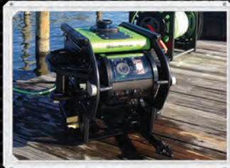
LBV300-5 versatile dual vertical thruster ROV system
