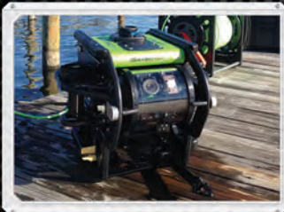
LBV300-5 versatile dual vertical thruster ROV system
