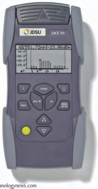
CWDM power meter.
