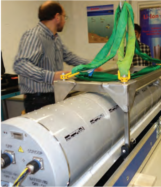
40kWh Li-Ion AUV battery, ready to be installed.
