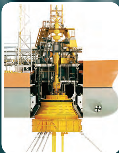
SBM Offshore FPSO Turret Mooring Syst.
