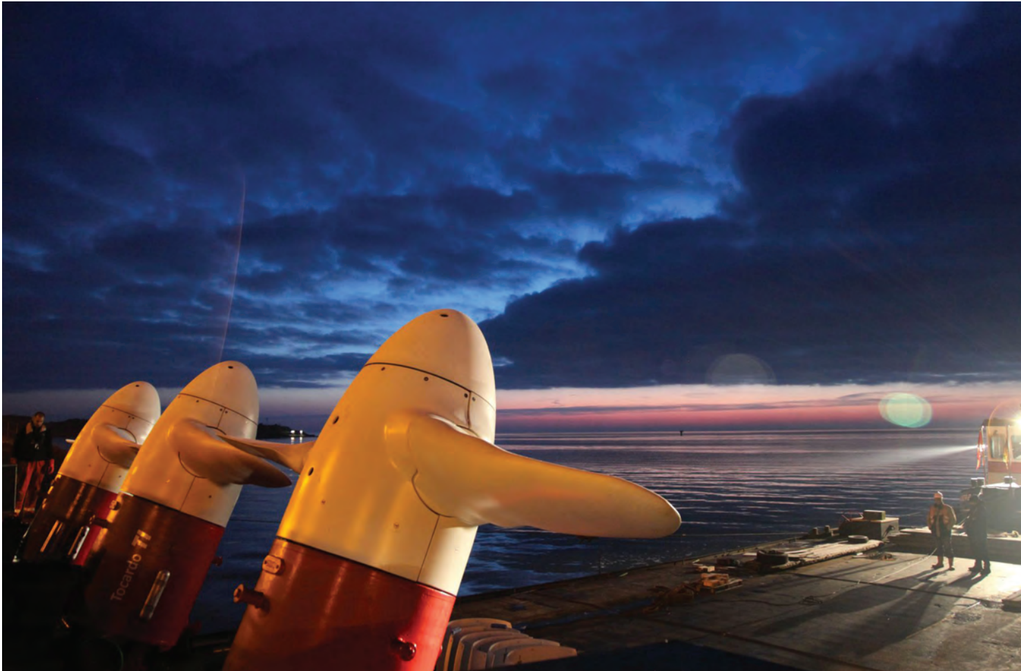
The Signature1000 is mounted on turbines that are installed in three different locations in the Netherlands. The TTC test facility in Den Oever, in the Eastern Scheldt storm surge barrier, and on the BlueTEC floating tidal Energy platform Texel.
