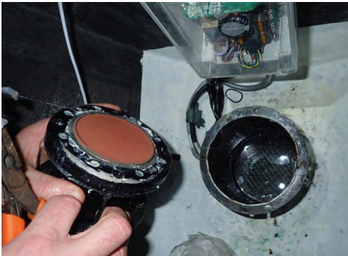
Above: Fig.4: The flat-faced phased array DVL was seated inside the carbon fiber hull. This location avoided adding hydrodynamic drag.
