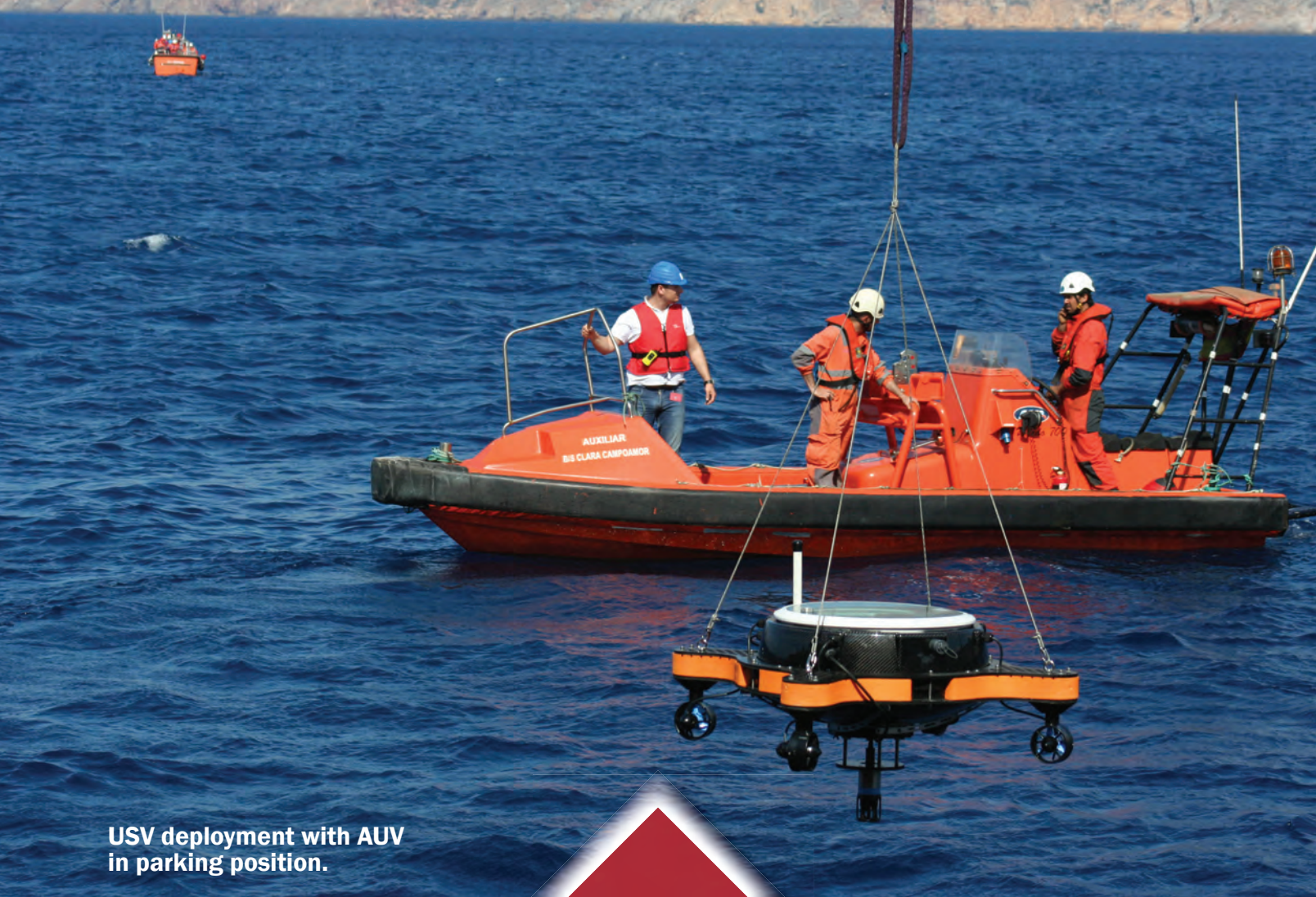
Deployment of the Remus 600 to join the rest of the fleet - 5 AUVs and 1 USV - to begin an unmanned multi-vehicle collaborative mission.
